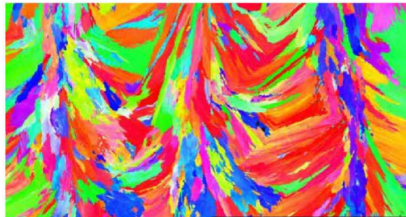
Image from electron backscattering diagnostic of grains in an additively-manufactured stainless steel. The different colors represent different grain orientations.
