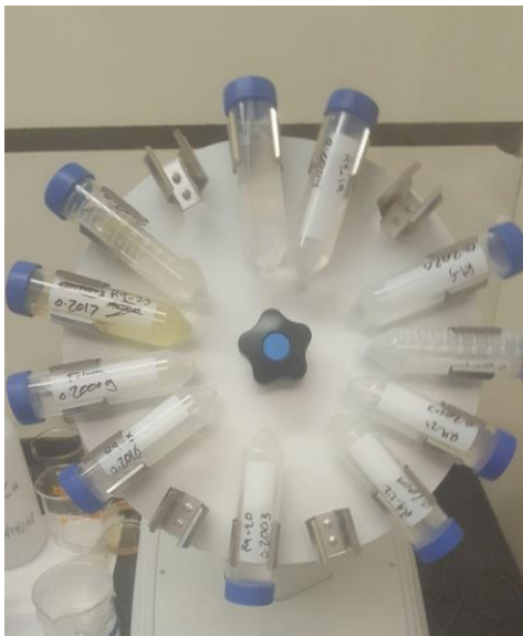
Figure 1. The Batch experiment consist of 50 ml tubes mounted on the rotator with Nd solution, Osorb, and Dipex.
