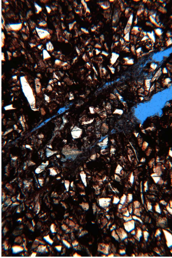
Plane light image of segmented macrofracture with abundant intragranular and transgranular microfractures in zone in between segments. Field of view = 2.043mm. Loading direction is vertical, sample MK2-2 C29 B2b.
