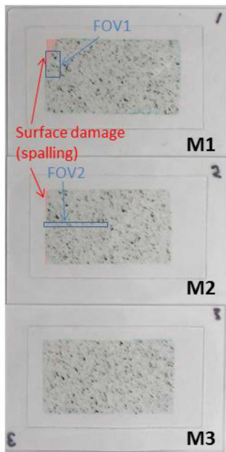
Figure 8.27. Petrographic thin section samples made for the Sections M1, M2, and M3 shown in Figure 3-19. The width of the samples is 50.8 mm, and the height 25.4 mm. Blue boxes (FOV1 and FOV2) in the figure indicate the field of view of the magnified microscope images shown in Figure 8.28.
