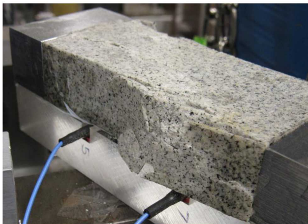
Figure 8.16. Side view of axial-splitting and buckling failure in Sample Z-3.
