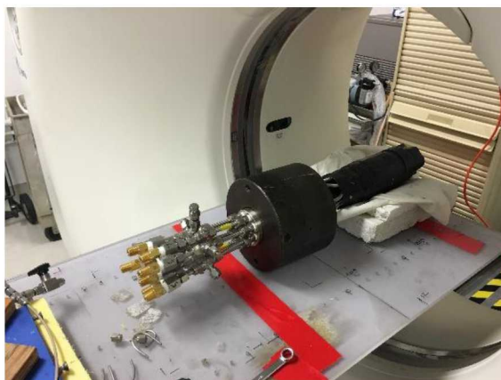
Figure 8.36. Sample on CT table ready for scanning.
