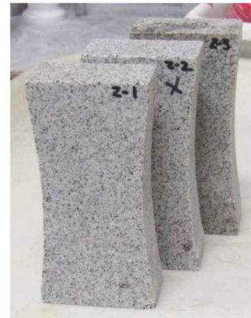
Figure 8.8. Photograph of shaped Westerly granite slabs used for the experiment.
