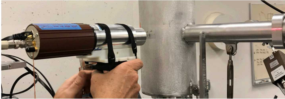
Alignment of the \text{LaBr}_3 detector at 95^\circ with respect to the ion beam
