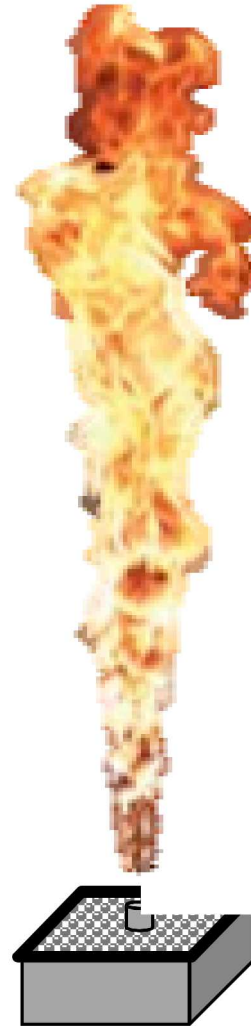
Fig. 9 LII image from a strongly turbulent jet flame
