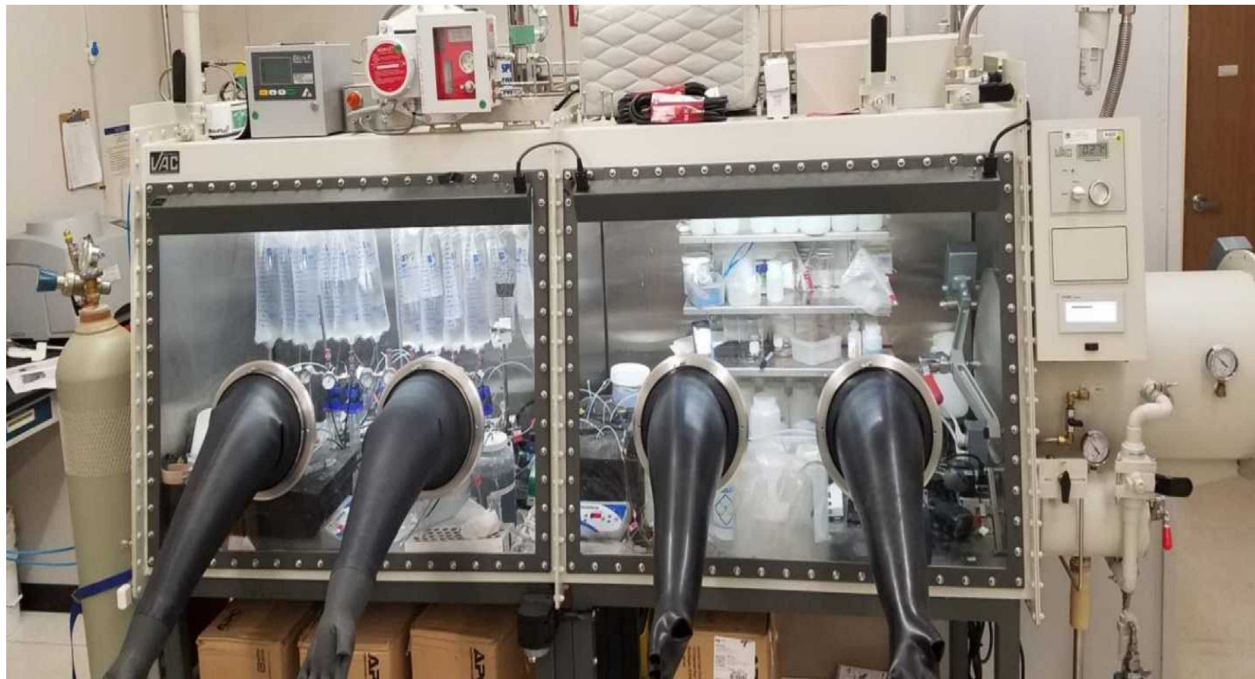
Figure 2. Glovebox setup for Single Pass Flow Thru Experiments. The hanging IV bags contain the experimental solutions. Reaction vessels are covered in insulating foam and cannot be seen.
