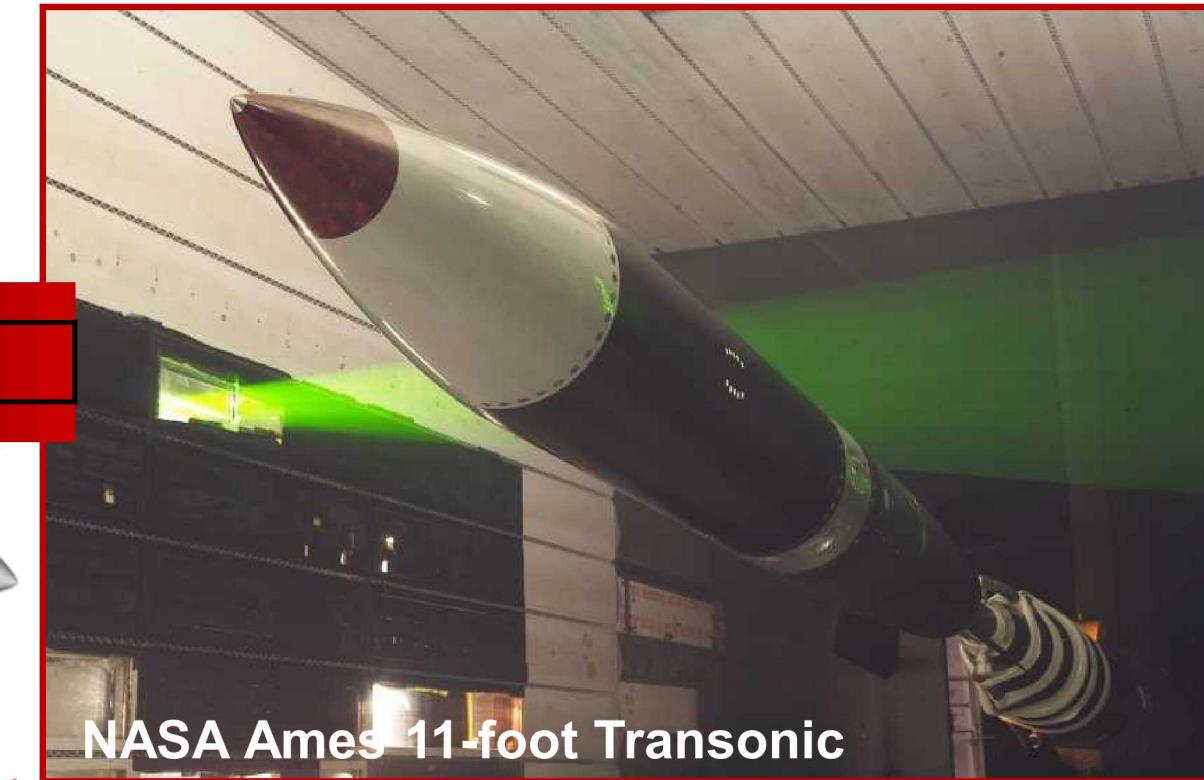
And we have successfully fielded PIV in large-scale production wind tunnels.
