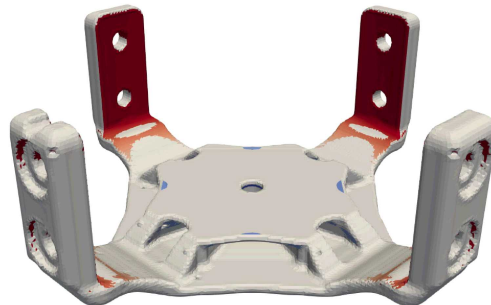
Design courtesy of Clinton Holtey using Plato. Displacement predictions by Kyle Johnson. Red = 0.1 mm.
