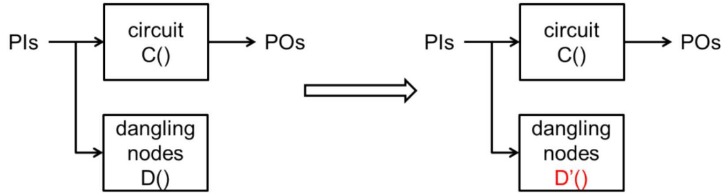
Figure 58. Dangling nodes are gates that do not appear on any path between the circuit's PIs and POs.
