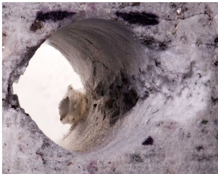
Figure 3.6: Closeup of borehole breakout in SWG generated with the SWESI geometry
