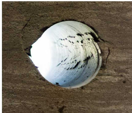
Figure 4.5 Sample PERP 1.2 after deformation. View shows fracture distribution along wellbore. The diameter of the undeformed borehole is 11.3 mm.
