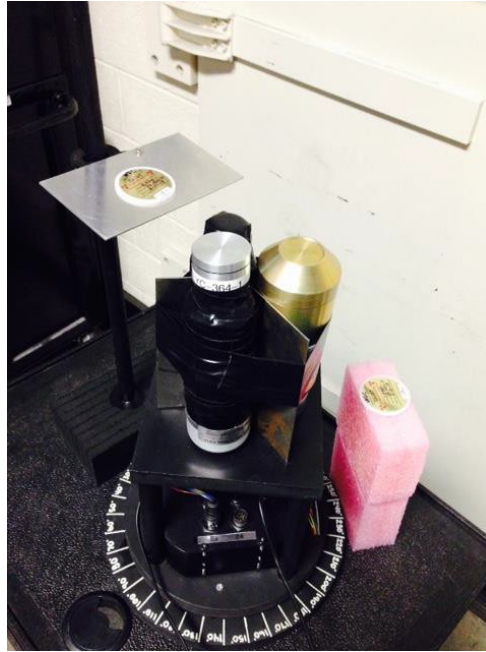
Figure 6. Two sources ( ^{137}\text{Cs} and ^{60}\text{Co} ): directional measurement experimental setup.
