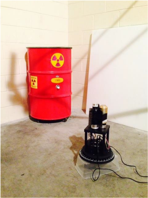
Figure 8. Directional measurements using a moderated ^{239}\text{PuBe} source.
