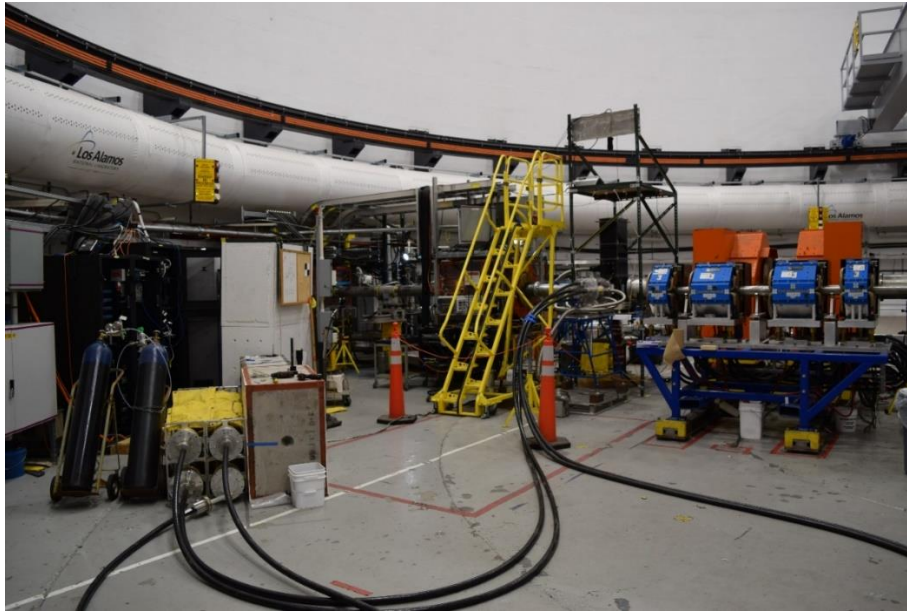
Figure 3.5. NNSS TDI multi-pulse flash x-ray system fielding setup at the LANL pRad facility. Four Marx generators, positioned in the lower left, are shielded from the beam line. Long, high-voltage cable transmission lines are shown connected to the x-ray diode head assembly in the experimental area in the pRad beam line.
