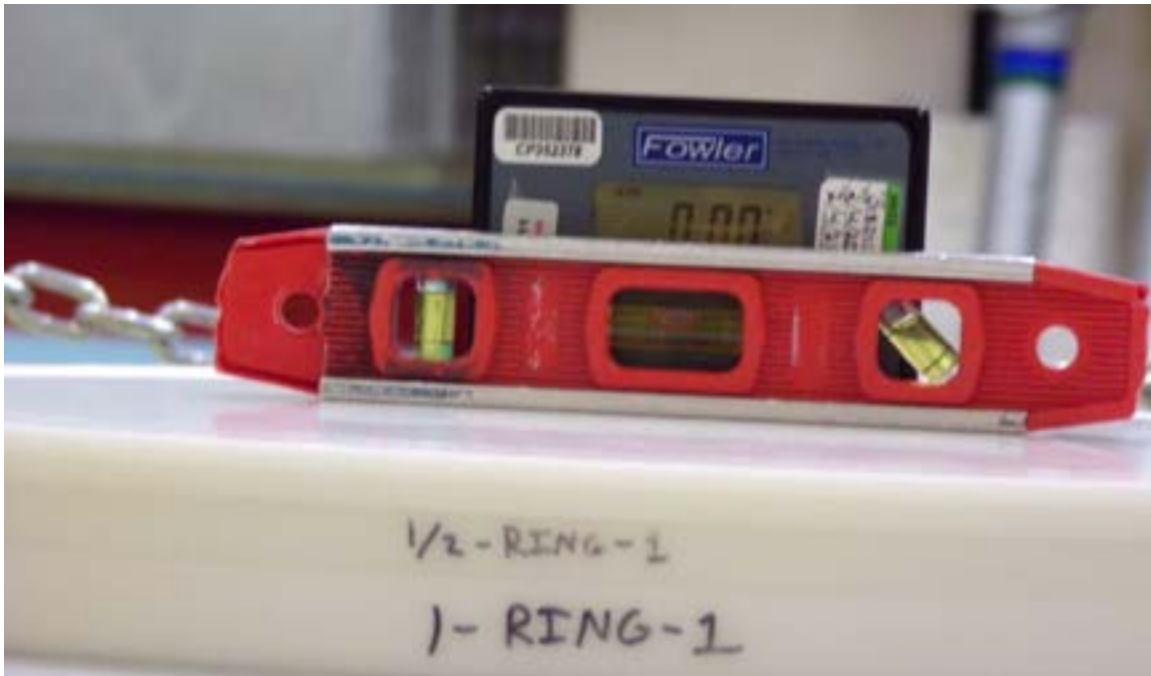
Figure 46: Levelness measurement for the upper half of the 0" experiment
