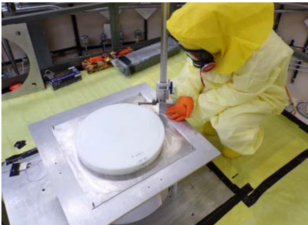
Figure 72: Operator performing overall height measurements for the upper half of the 1/2" experiment.
