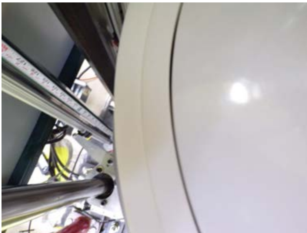
Figure 31: Close-up of the gap between the reflector rings and plate stack.
