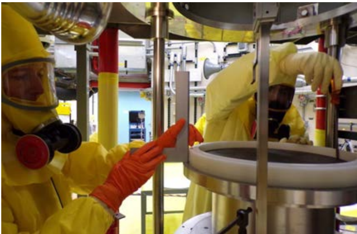
Figure 32: Operators using a T-square to align the first reflector ring with the bottom reflector and a tool to push the stack to one side of the reflector rings.
