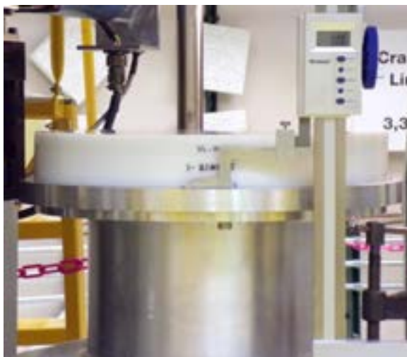
Figure 39: Height gauge measuring the overall stack height of the lower half of the experiment where it must be zeroed on the lip of the lower adapter plate.
