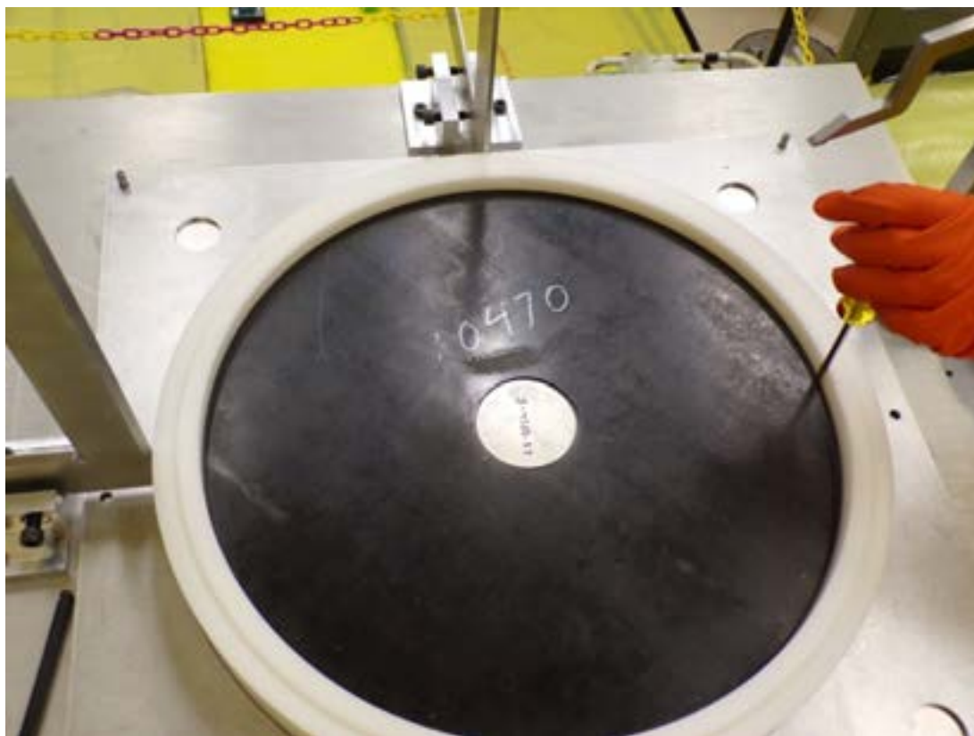
Figure 27: HEU and moderator plate stack alignment within the reflector rings, showing an operator using a tool to push the stack to one side of the reflector rings.
