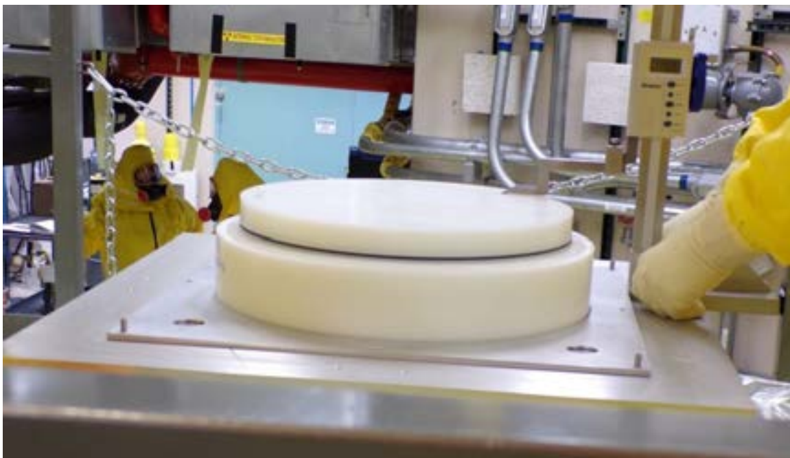
Figure 85: Upper half of the 1½” configuration with ring reflectors around the fuel and moderator stack, but not yet around the top reflectors.
