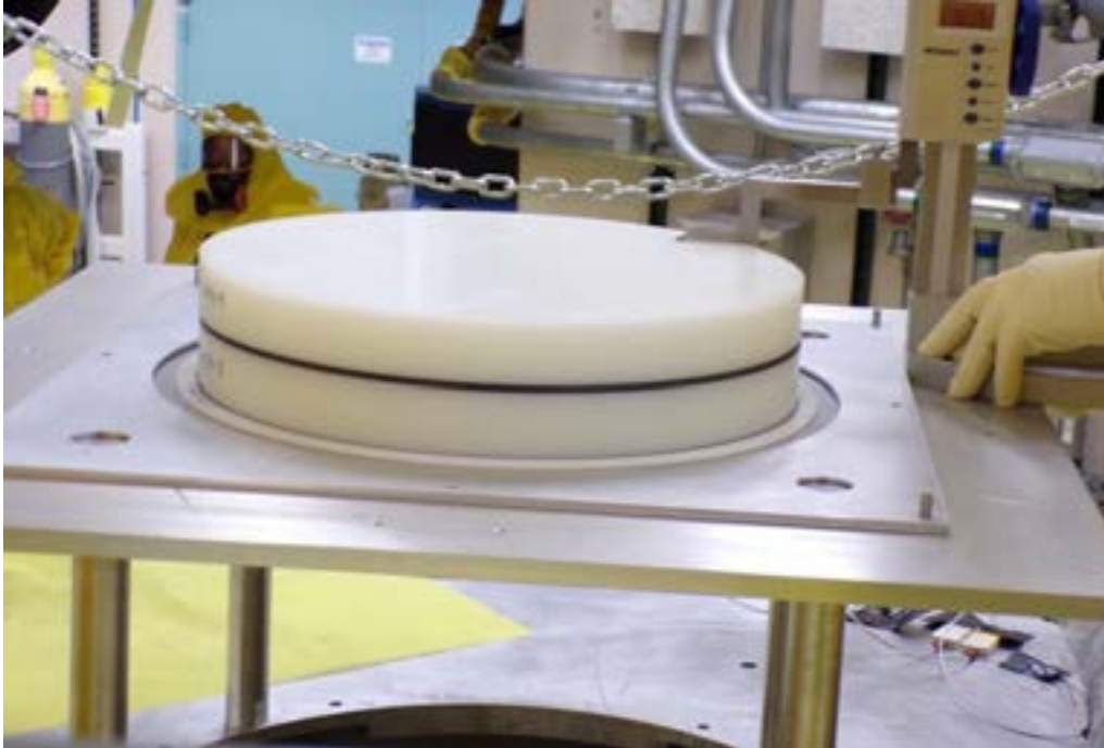
Figure 84: Partial upper half of the 1½” experiment, showing 2 HEU plates and 2 moderator plates along with the alignment plate atop the membrane.
