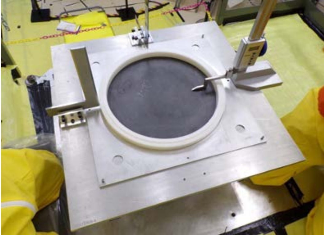
Figure 50: Height measurement of the first HEU plate on the upper half of the \frac{1}{8} " B experiment.
