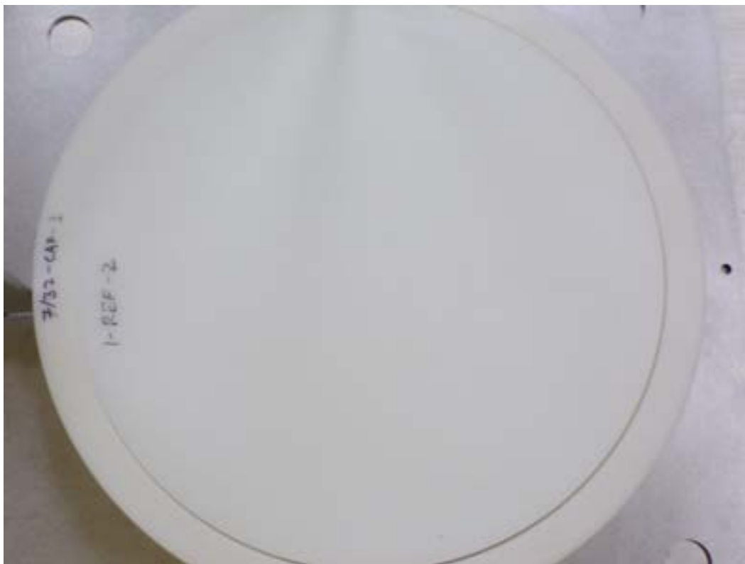
Figure 30: Gap between the reflector rings and the plate stack.
