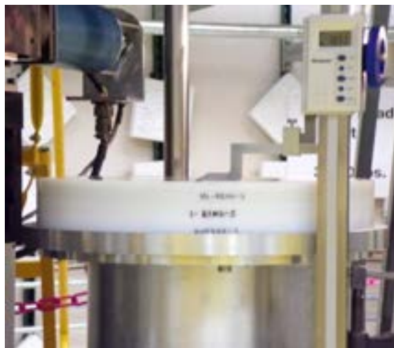
Figure 39: Height gauge measuring the overall stack height of the lower half of the experiment where it must be zeroed on the lip of the lower adapter plate.
