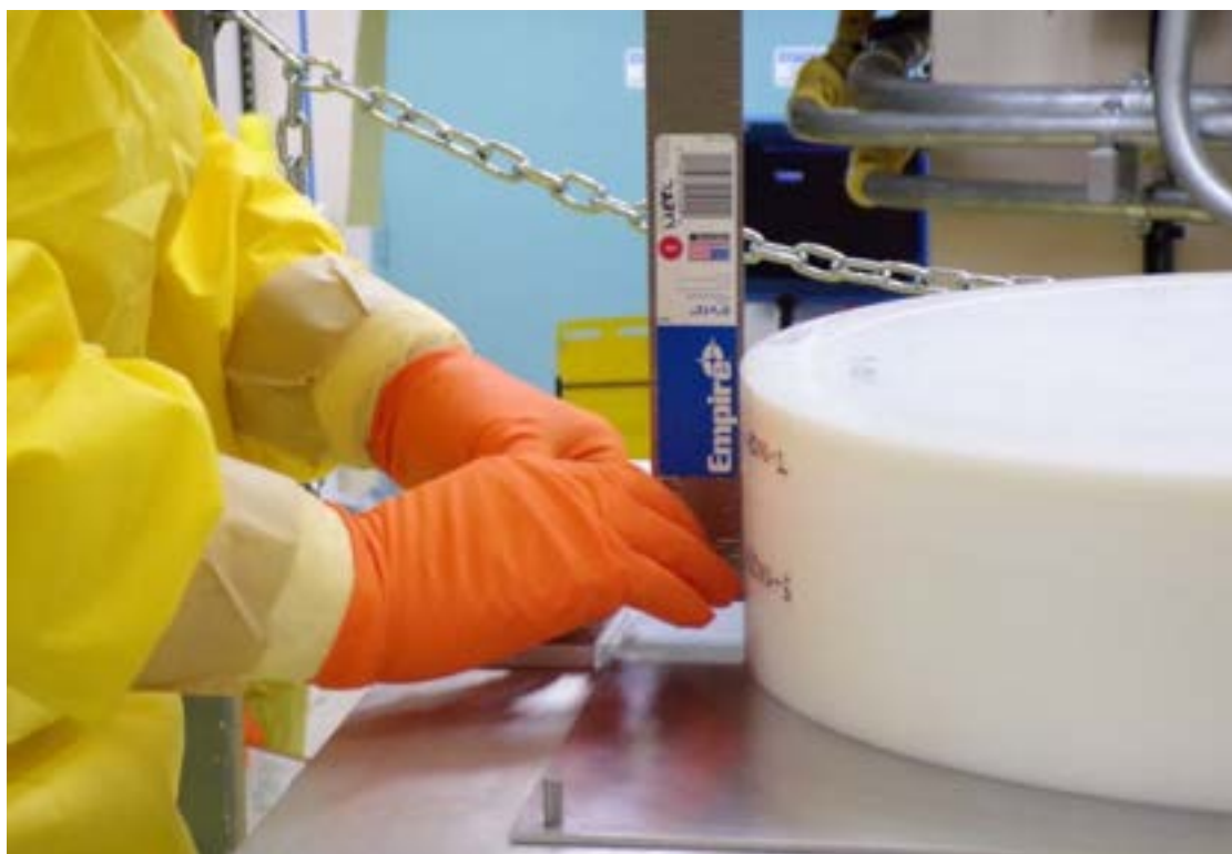
Figure 34: Operator using a T-square for final alignment of the reflector rings.
