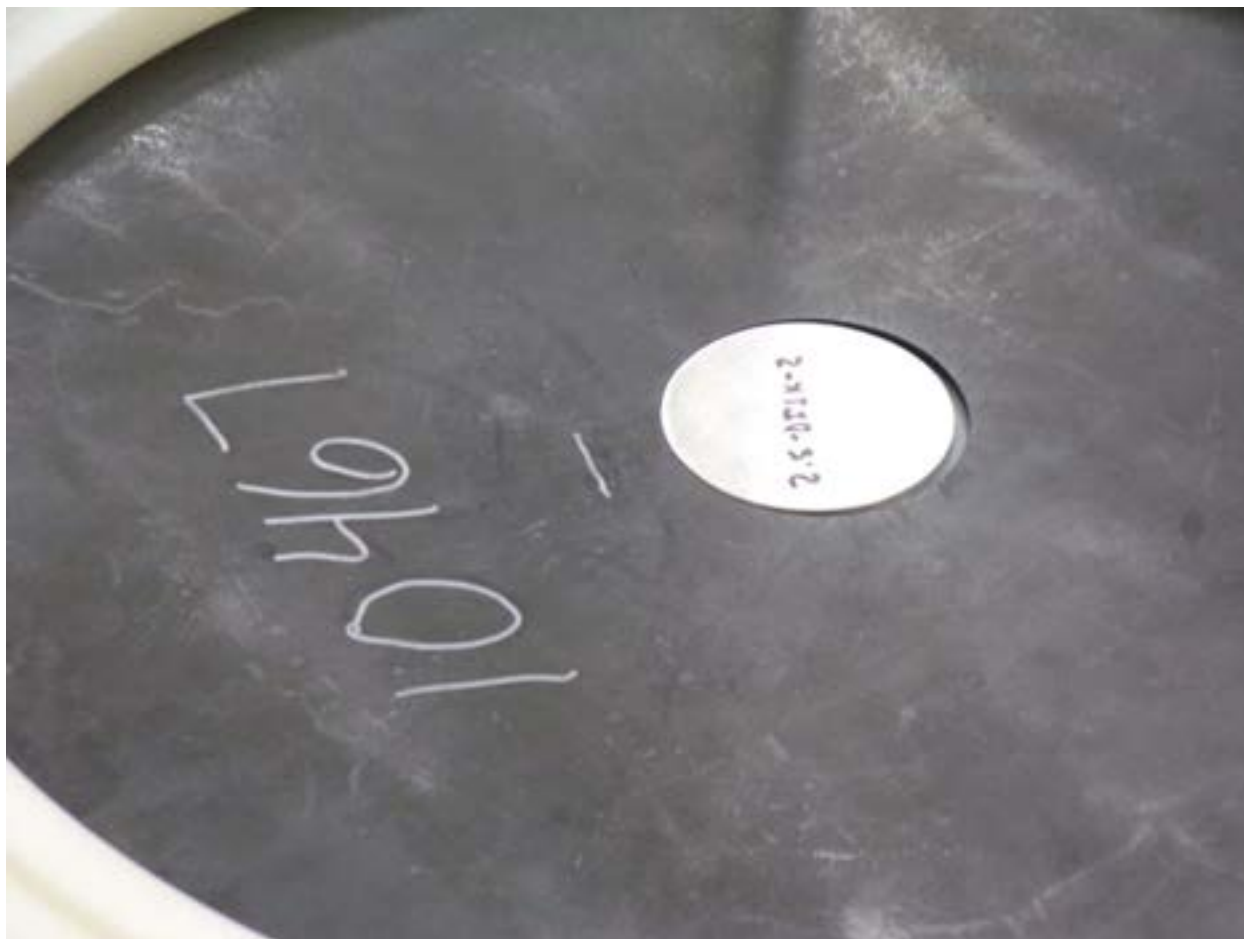
Figure 28: Insert in an HEU plate with a 2.5" annulus, showing the insert pushed to the same side as the plate.
