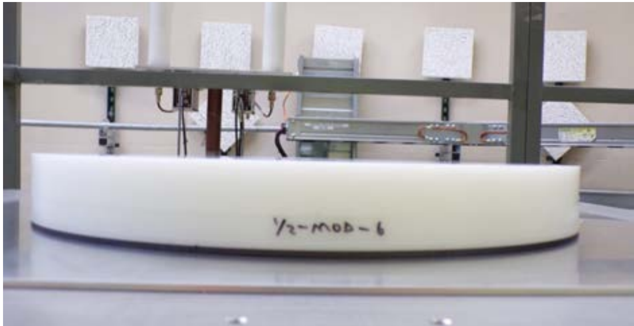
Figure 77: Upper half of the \frac{1}{2} " configuration with ring reflectors removed during disassembly. The 1/2-MOD-6 moderator plate is used as a reflector.
