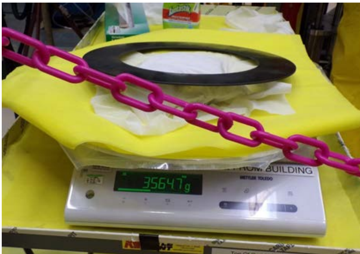
Figure 11: Mass measurement of HEU plate with 10" annulus (10479).
