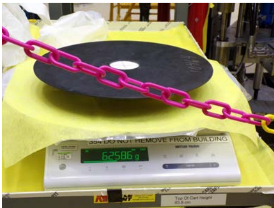
Figure 9: Mass measurement of HEU plate with 2.5" annulus (10464).
