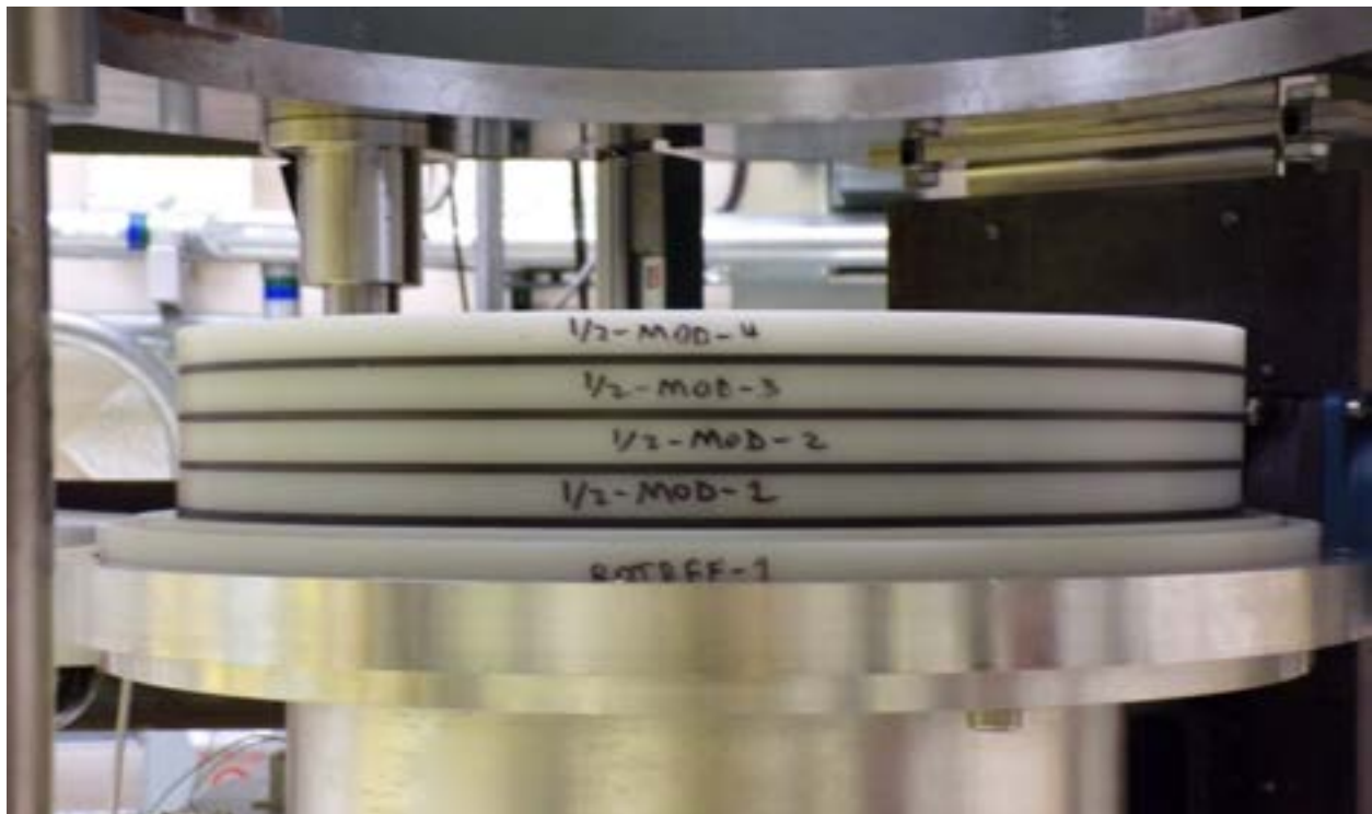
Figure 78: Lower half of the \frac{1}{2} " configuration with ring reflectors removed during disassembly, showing all moderator part IDs.
