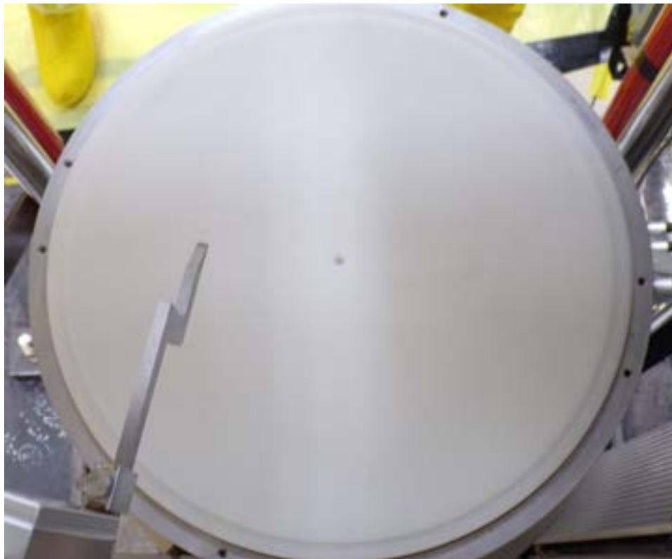
Figure 23: Top-down view of the reflector base, showing the neutron source cavity.
