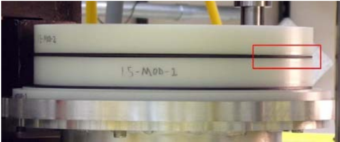
Figure 92: Moderator plate (1.5-MOD-2) not sitting flush with the HEU plate (10493).
