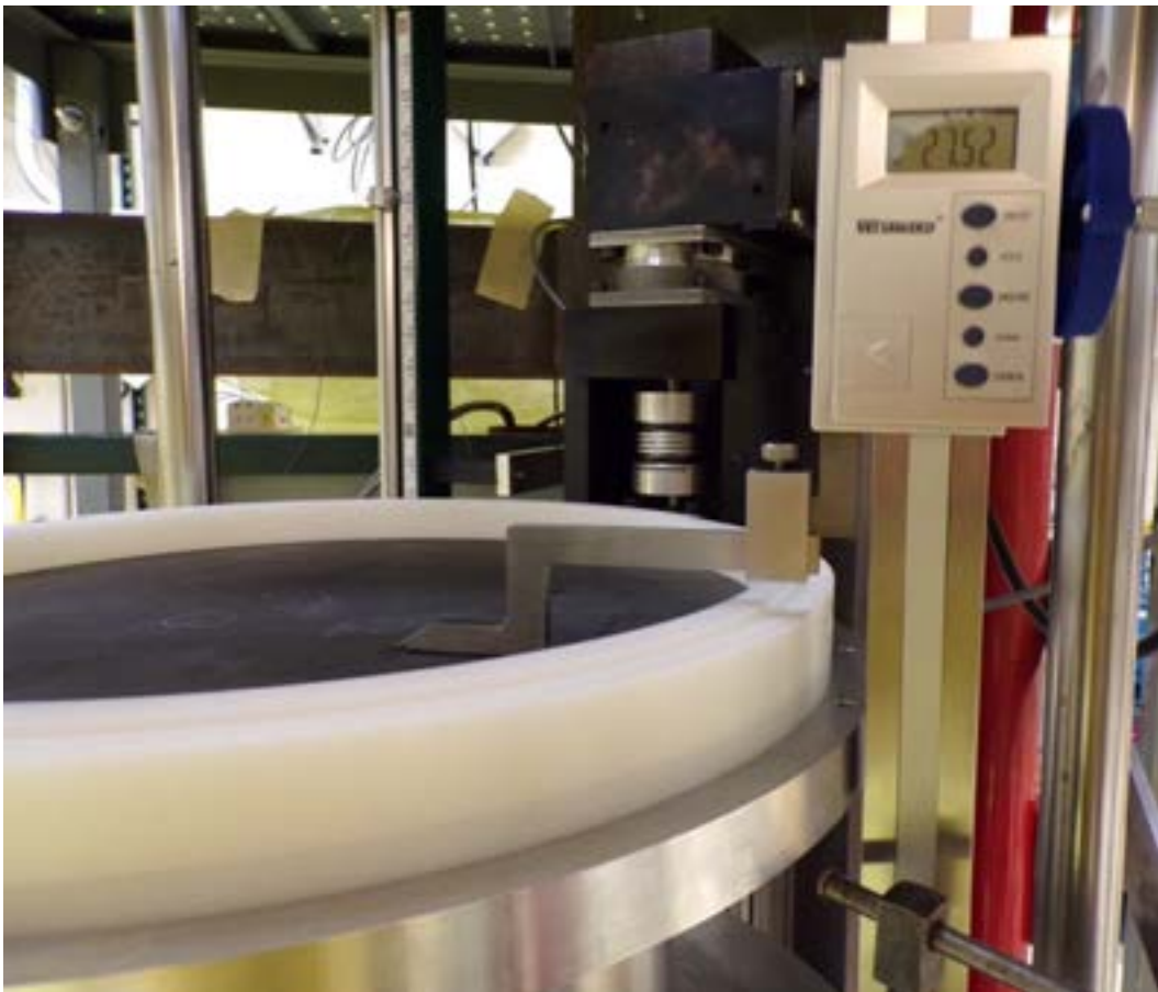
Figure 61: Height measurement of an HEU plate (11150) on the lower half of the 1/4" experiment.
