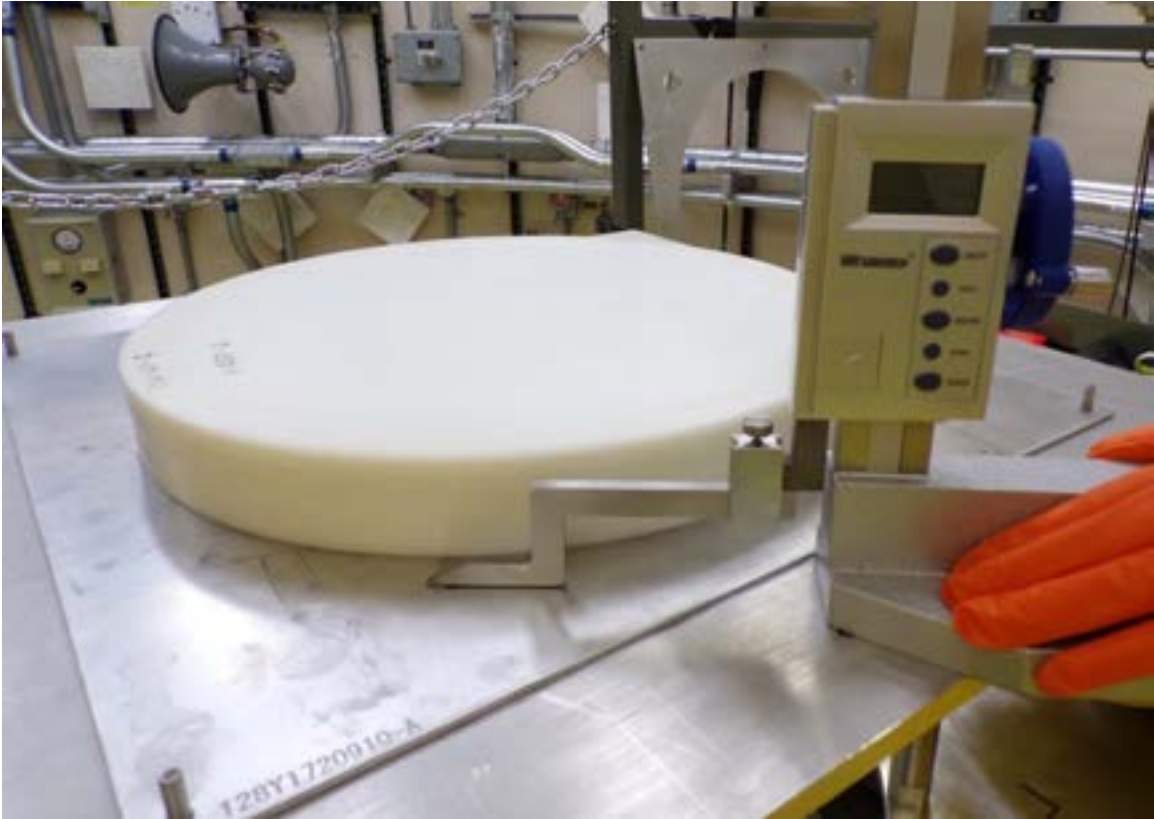
Figure 52: Zeroing the height gauge for the overall height measurement of the upper half of the \frac{1}{8} " A experiment.
