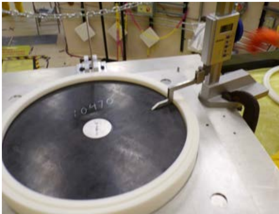
Figure 36: Height gauge clamped to the interface plate for height measurements of the upper half of the experiment.
