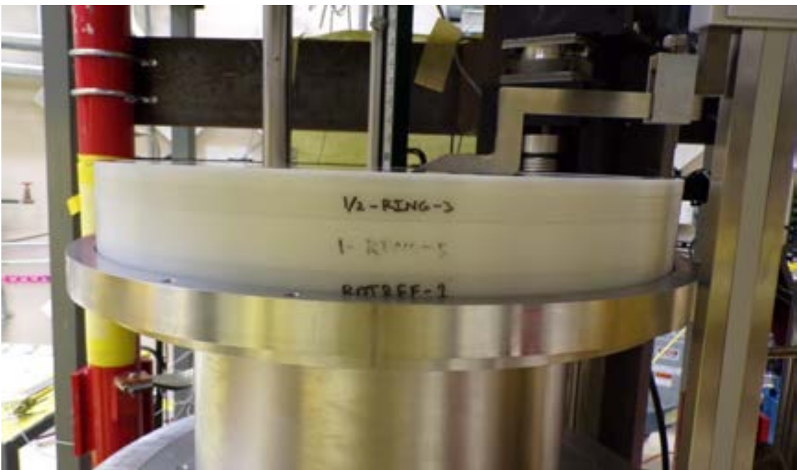
Figure 53: Overall height measurement of the lower half of the \frac{1}{8} " experiment (used by both \frac{1}{8} " A and \frac{1}{8} " B).
