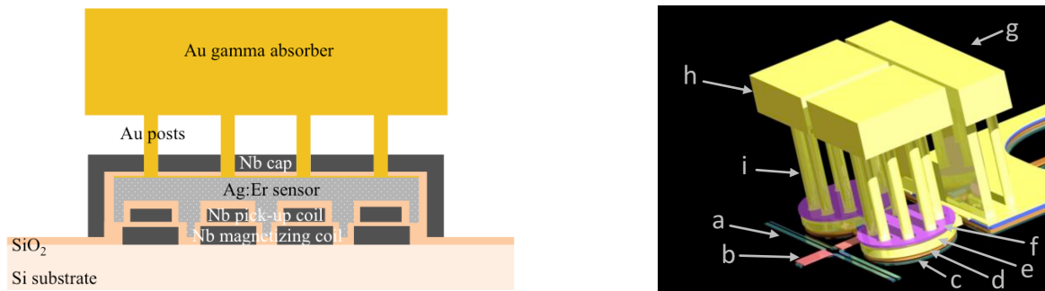
Figure 1 (left): Schematic cross-section of an MMC gamma detector (not to scale). The thick electroplated \gamma absorber is supported on top of the paramagnetic Ag:Er sensor by Au posts. The lower Nb coil is used to magnetize the sensor, and the upper coil is used to pick up the signal and couple it to the SQUID preamplifier. Figure 2 (right): A 3D schematic of an MMC shows the magnetizing circuit (a), the heat switch (b) to trap the current in the magnetizing coil (c), the sensing coil (d) below the paramagnetic Ag:Er sensor (e), the superconducting Nb cap (f) to confine the magnetizing field to the sensor (e), and the Au absorber (h) supported on Au posts (i, with height greatly exaggerated for clarity) on top of the sensor. The thermal bus (g) is designed to efficiently cool the MMC back to the base temperature of the cryostat [Boyd 2018].
