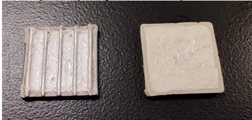
Figure 3.9. Finned and flat PZT ceramics fabricated through the ME process after sintering with coated silver electrodes.
