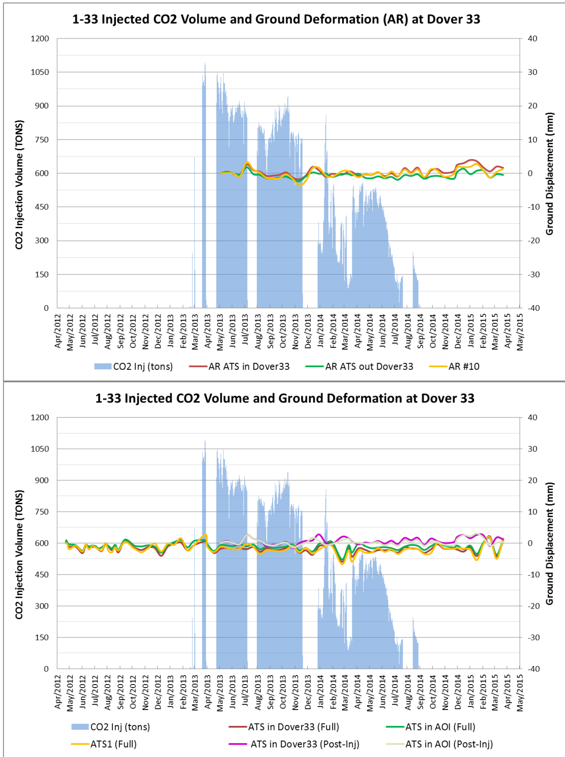
Figure 54: Injected CO 2 volume and ground deformation results obtained at Dover 33. The top panel represents ground deformation results obtained from the ARs, while the bottom panel shows ground deformation results obtained from natural radar targets for both the full and co-injection data.
