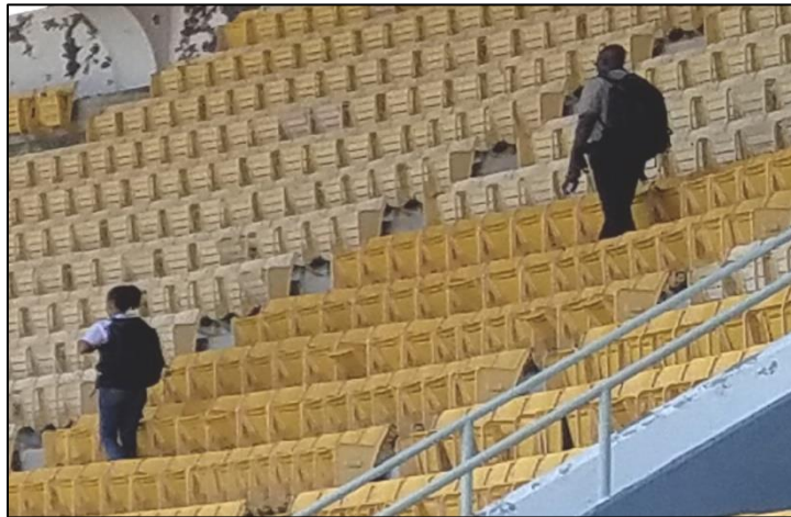
FIG 3. Backpack detector baseline search/survey of a stadium prior to an MPE using an optimized grid search pattern.
