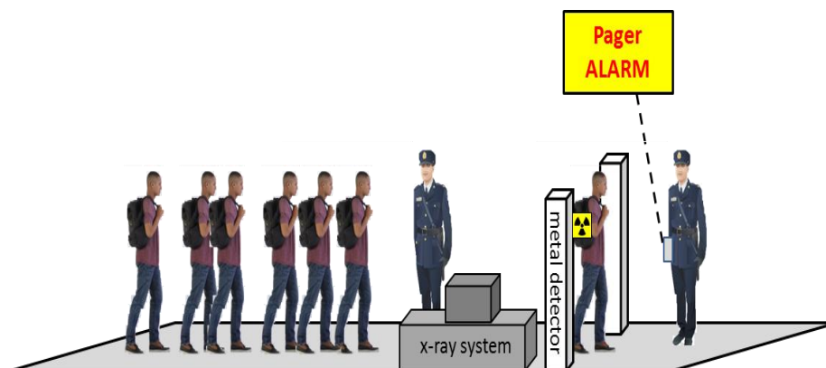
FIG 2. Examples of an MPE checkpoint with a magnetometer, an x-ray machine, and a security officer with a radiation pager.
