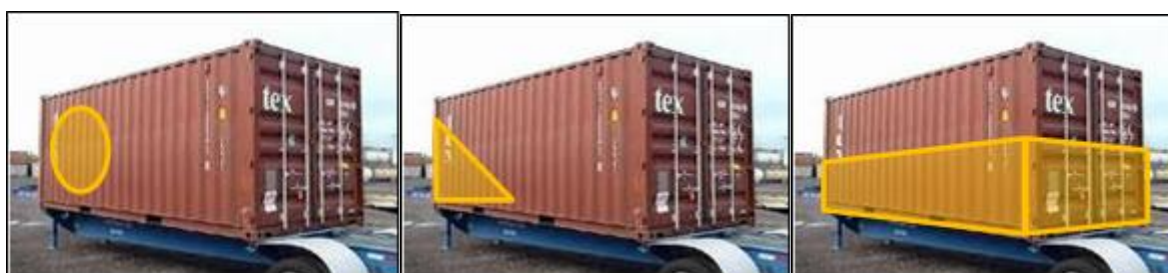
FIG 3. Radiation signatures of point (left), distributed (center) and uniformly distributed (right) sources in cargo containers.
