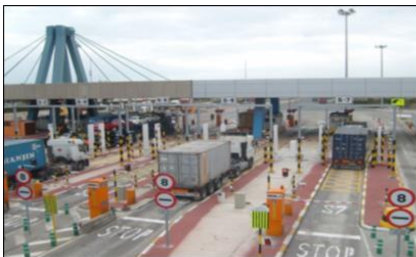
FIG 1. Radiation portal monitor system to scan cargo containers at a shipping port.
