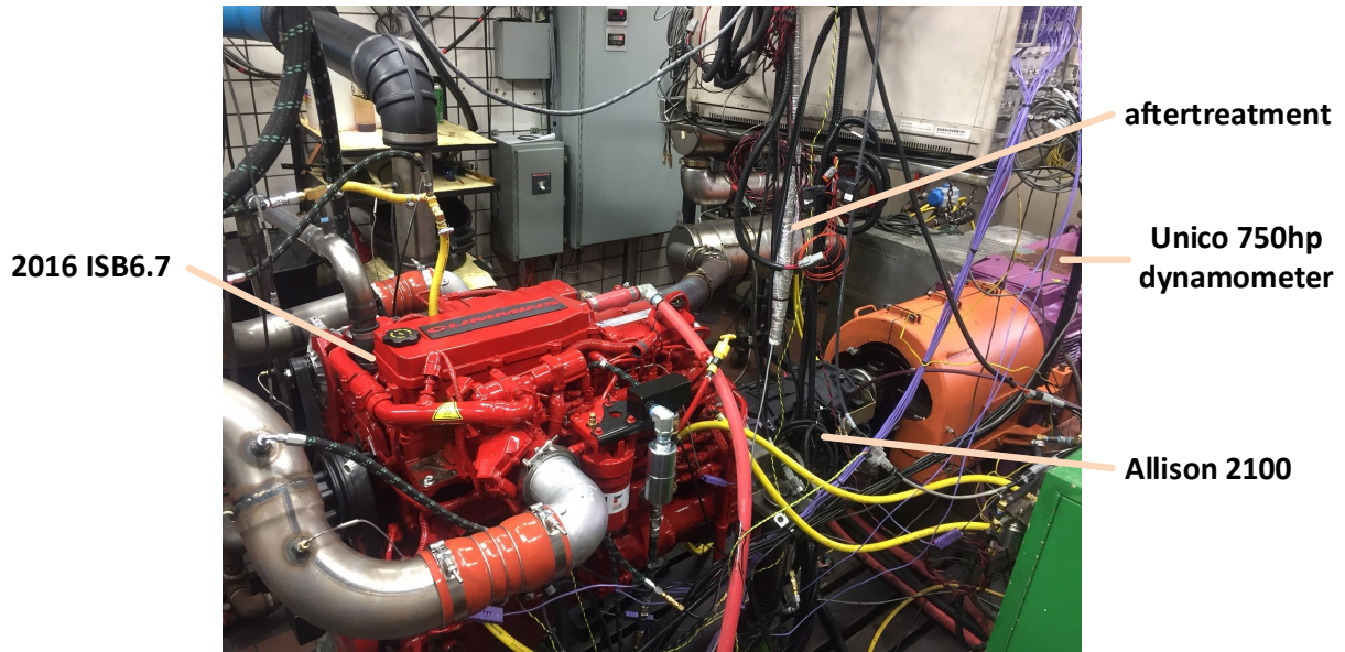
Figure 13: Conventional Powertrain in Cummins Test Cell
