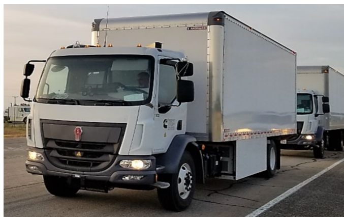
Figure 3: ETREE vehicle(front) and conventional diesel vehicle staged for J1526 testing
