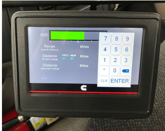
Figure 6: Human Machine Interface for Daily Mileage Entry
