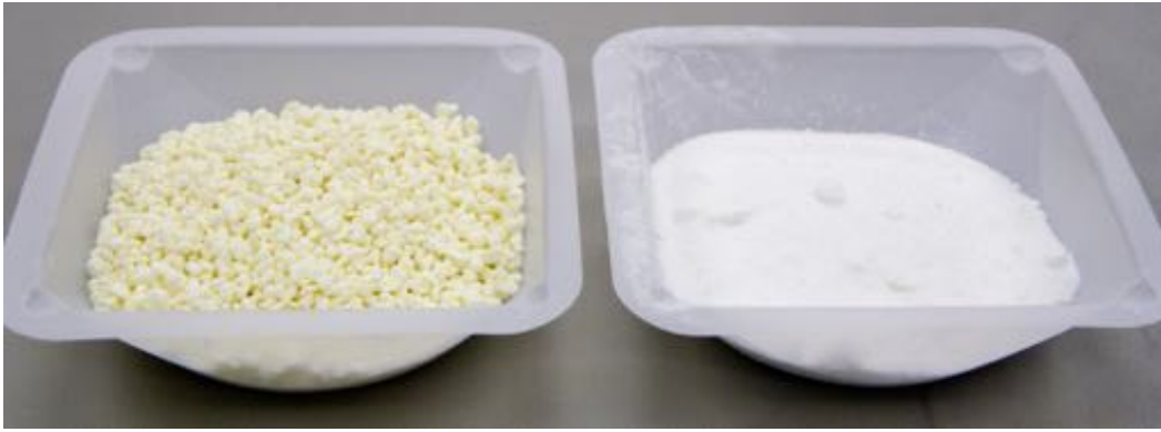
Figure 1. Photos of PBX 9501 molding prills (left) and Class 1 HMX powder (right).
