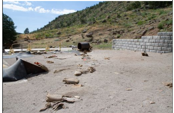
Figure 39. Test 3, 10 inch prills, post-shot. Shot stand obliterated (original location was at middle pile of sandbag garbage).
