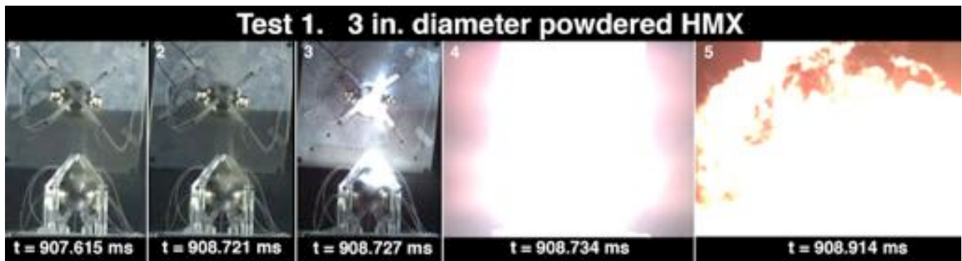
Figure 18. Test 1, Phantom video. 3 inch powdered HMX. Frame 1 and 2 show smoke escaping from between the shells. Frame three is the first frame with light. Frame 4 is the next captured image, \approx 6 \mu\text{s} later. Frame 5 shows the late-time fireball.
