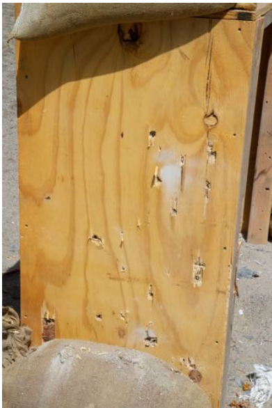
Figure 36. Test 1 post-shot, showing fragment penetrations through 3/4 inch plywood.
