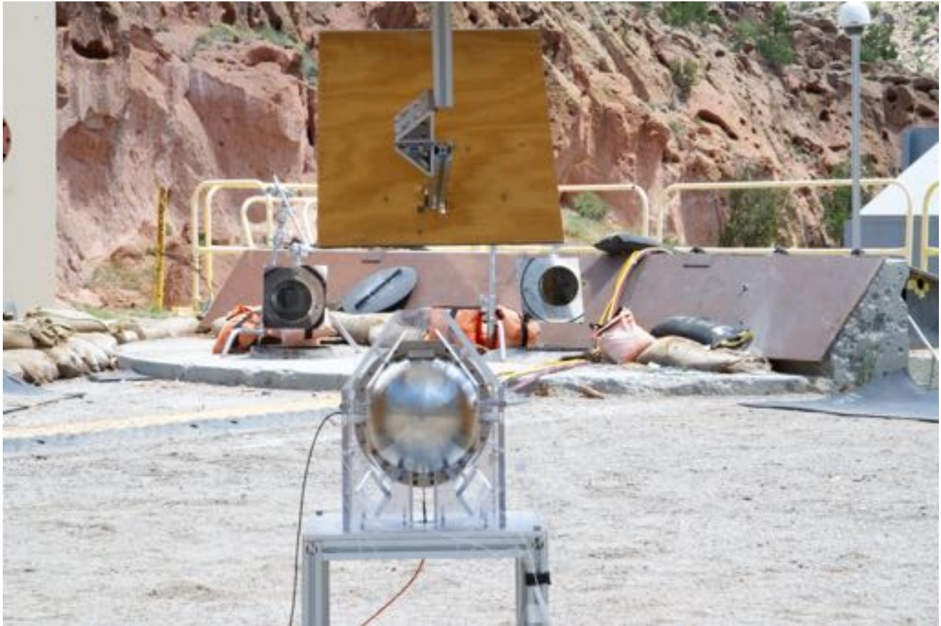
Figure 17. Photograph from a viewpoint behind the shot for Test 5, looking back at the turning mirrors located above the portholes in the bunker. The Phantom camera observes through the porthole on the left of the image; the Shimadzu through the right. Also visible is the turning mirror situated directly above the shot, which provides a top-down view of the shot.
