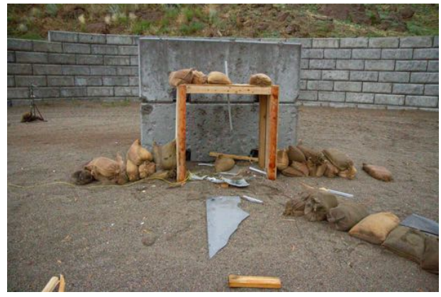
Figure 49. Test 7, post-shot. Shot stand damaged but not completely obliterated.
