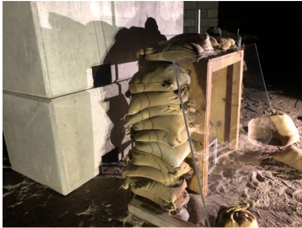
Figure 44. Test 7, pre-shot. Additional mitigation for fragment fire prevention is shown. A 1-inch thick polycarbonate sheet is leaned against the front of the stand. Note that mitigation blocks blast gauge line-of-sight to the shot.
