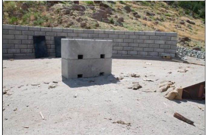
Figure 45. Test 7, post-shot. All parts of mitigation (excepting blocks) were obliterated.
