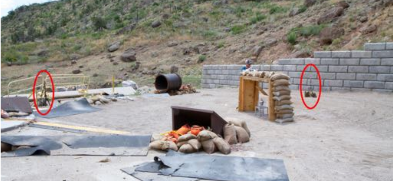
Figure 16. Photograph of site layout, Test 5. Blast gauges are mounted to metal tripod stands on far right ("south") and left ("east") of the image, circled in red. Metal blast shield in foreground serves as protection for the final optical coupler box. The wooden arch and sandbags are intended to catch the larger fragments that might form from the thicker flange portion of the metal shells, in the event of a violent reaction.
