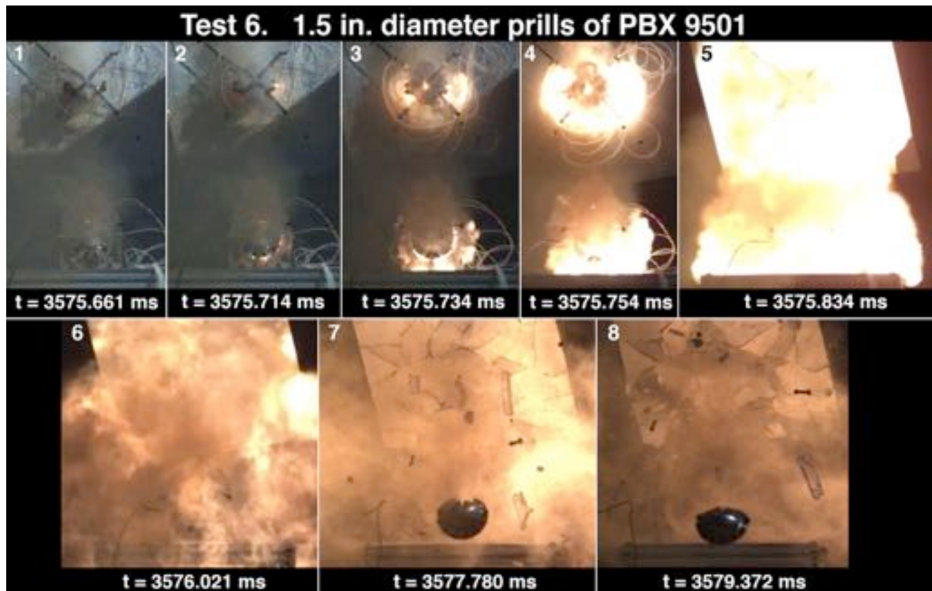
Figure 28. Test 6, Phantom video. 1.5-inch diameter PBX 9501 prills. In frames 7 and 8 a mostly intact hemisphere is visible.
