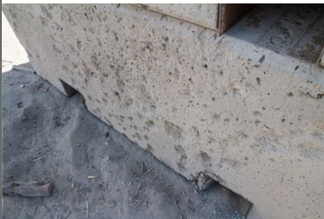
Figure 46. Test 7, post-shot. Pitting of concrete block was caused by stainless fragments from the case.
