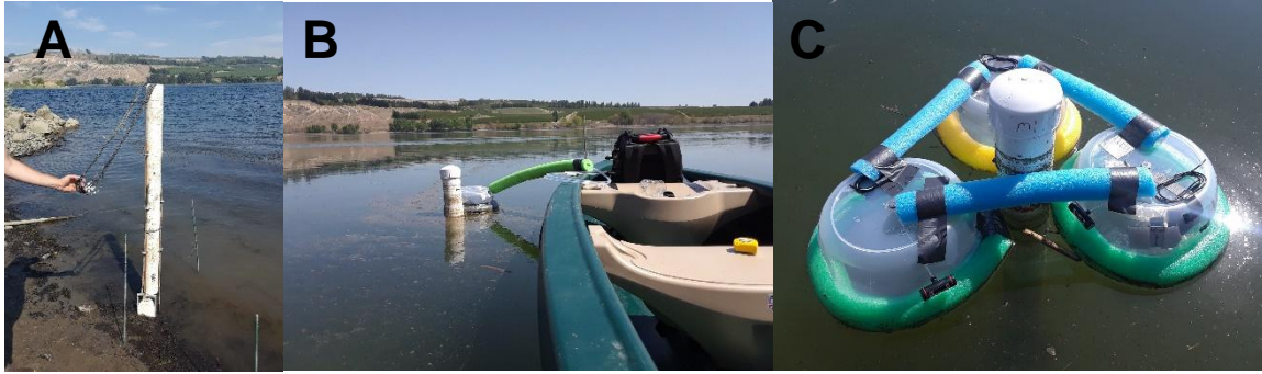
Figure 1. Chamber positioning approach. (A) installed peeper (below ground) with white PVC conduit extending above the peeper location held up by 3 rebar rods (inside the conduit, not visible in picture). The PVC conduit houses the sampling tubing (in the picture, the tubing is extended to full length beyond the top end of the PVC tube and held by Dr. Villa's hand). (B) positioning and securing of the methane sampling chamber above the peeper location as marked by the PVC conduit. (C) positioning and anchoring of the N 2 O sampling chambers, surrounding the PVC conduit around the peeper location.
