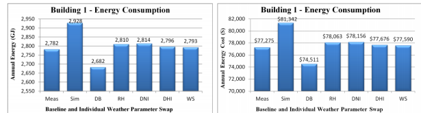
Figure 2: Dry bulb temperature, on average, tends to dominate changes in building energy use as shown here for DOE's Medium Office reference model. The next most important meteorological variables tend to be relative humidity, direct normal incident radiation, direct horizontal incident radiation, and wind speed.
