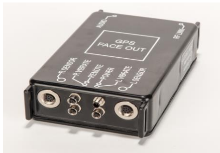
Radiation Backpack Control Panel
