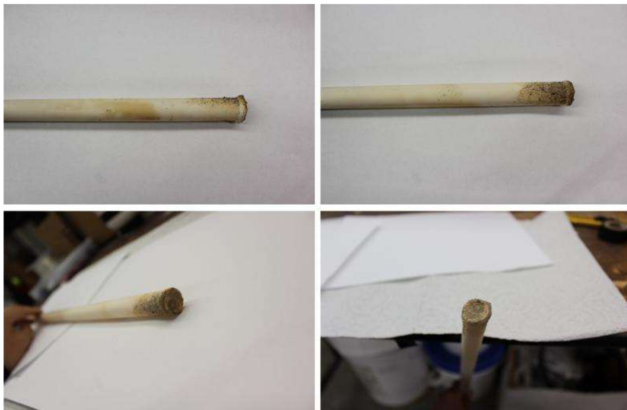
Figure. 52 Images of the sensor after 20 h operation in the Longview's utility boiler.
