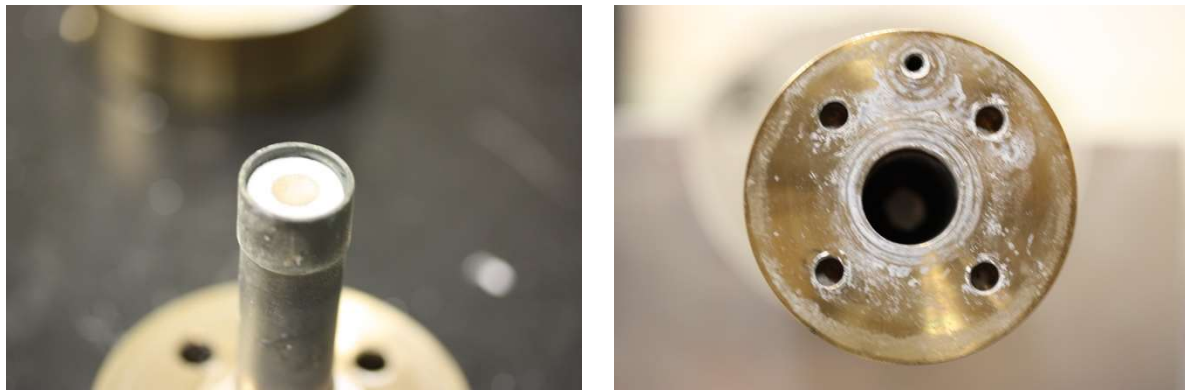
Figure 8: (upper left) Overall view of the process probe of length determined by boiler application. (upper right) The electrochemical cell, metal gasket and protective porous cap. (center left) Photograph of the reference electrode side of the YSZ-based oxygen cell. (center right) Looking down the bore axis of the process probe showing ceramic rod that picks up signal from the reference electrode. The interior volume is swept continuously with reference gas (air) to fixed oxygen chemical potential at the reference electrode. (lower left) gas
