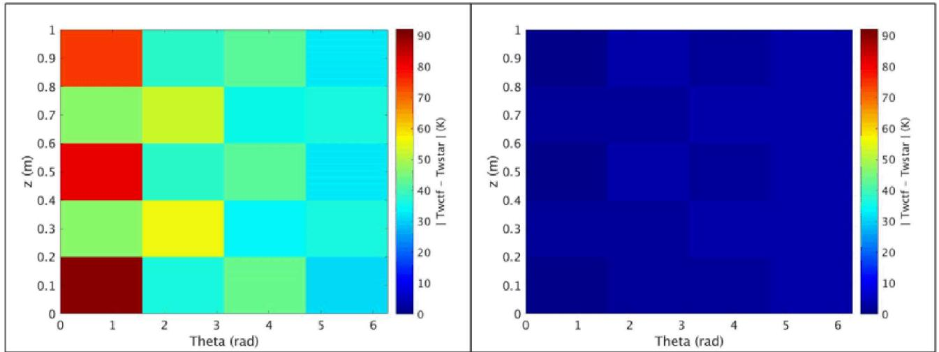
**Figure 7:**  $|\bar{T}_{w,CTF-post} - \bar{T}_{w,STAR,MMS}|$  plotted before calibration (left) and  $|\bar{T}_{w,CTF-post} - \bar{T}_{w,STAR,MMS}|$  plotted after calibration (right) for one manufactured dataset without noise.
