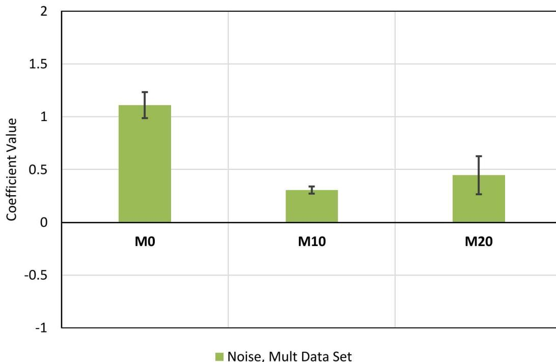
**Figure 10: Graphical representation of the optimal values and standard deviation for the M coefficients based on a calibration of 21 manufactured datasets with noise. The confidence intervals are narrower since 21 sets of data were used to calibrate the three parameters.**
