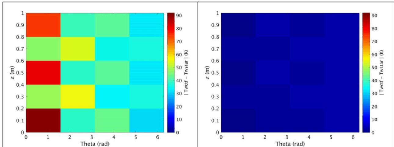
**Figure 9:  $|\bar{T}_{w,CTF-post} - \bar{T}_{w,STAR,MMS}|$  plotted before calibration (left) and  $|\bar{T}_{w,CTF-post} - \bar{T}_{w,STAR,MMS}|$  plotted after calibration (right) for one manufactured dataset with noise.**
