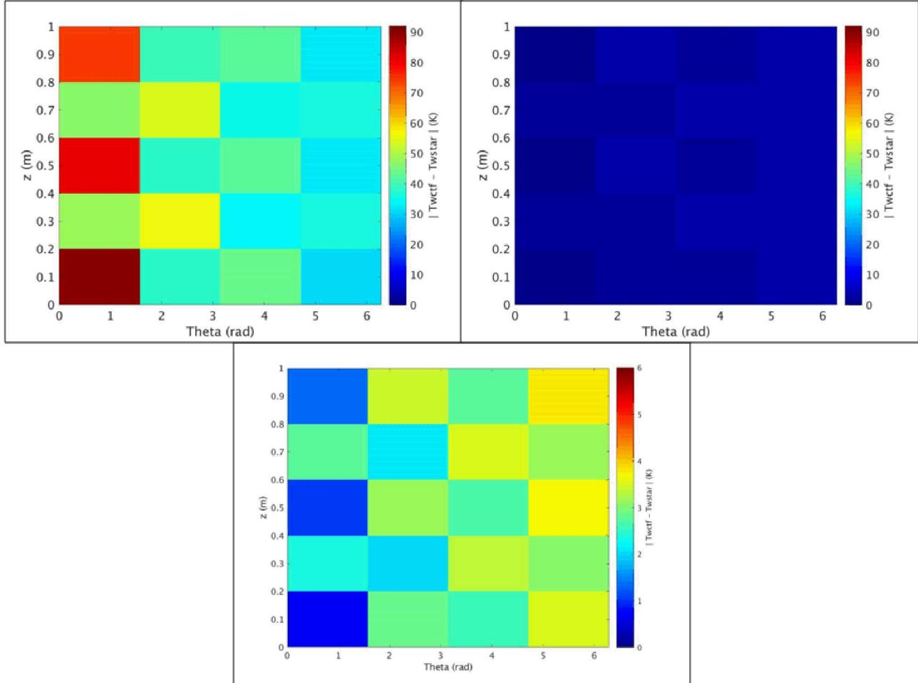
**Figure 11:**  $|\bar{T}_{w,CTF-post} - \bar{T}_{w,STAR,MMS}|$  plotted before calibration (top left),  $|\bar{T}_{w,CTF-post} - \bar{T}_{w,STAR,MMS}|$  plotted after calibration (top right), and  $|\bar{T}_{w,CTF-post} - \bar{T}_{w,STAR,MMS}|$  plotted on a narrower scale (bottom) for 21 manufactured datasets with noise.
