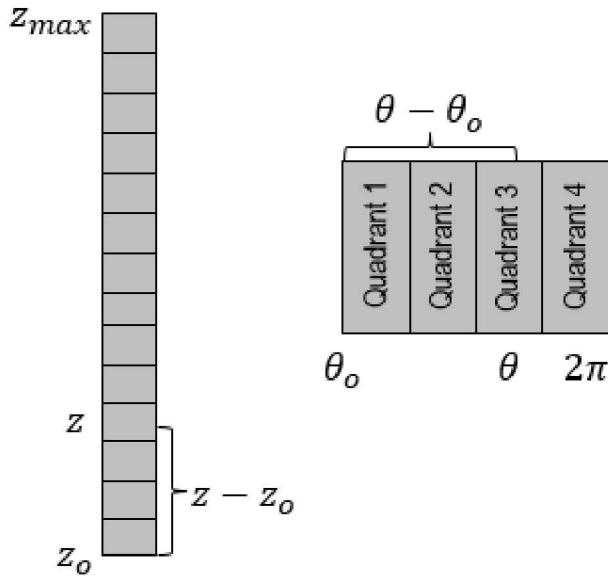
**Figure 1: A graphical explanation of  $z - z_o$  and  $\theta - \theta_o$  for any given  $z$  less than  $z_{max}$  and  $2\pi$  respectively. Regardless of specified geometry, CTF always outputs rod values in terms of four quadrants.**
