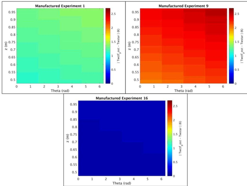
**Figure 16:**  $|\bar{T}_{w,CTF-post} - \bar{T}_{w,STAR}|$  plotted after calibration for Experiment 1 (top left),  $|\bar{T}_{w,CTF-post} - \bar{T}_{w,STAR}|$  plotted after calibration for Experiment 9 (top right), and  $|\bar{T}_{w,CTF-post} - \bar{T}_{w,STAR}|$  plotted for Experiment 16 (bottom).
