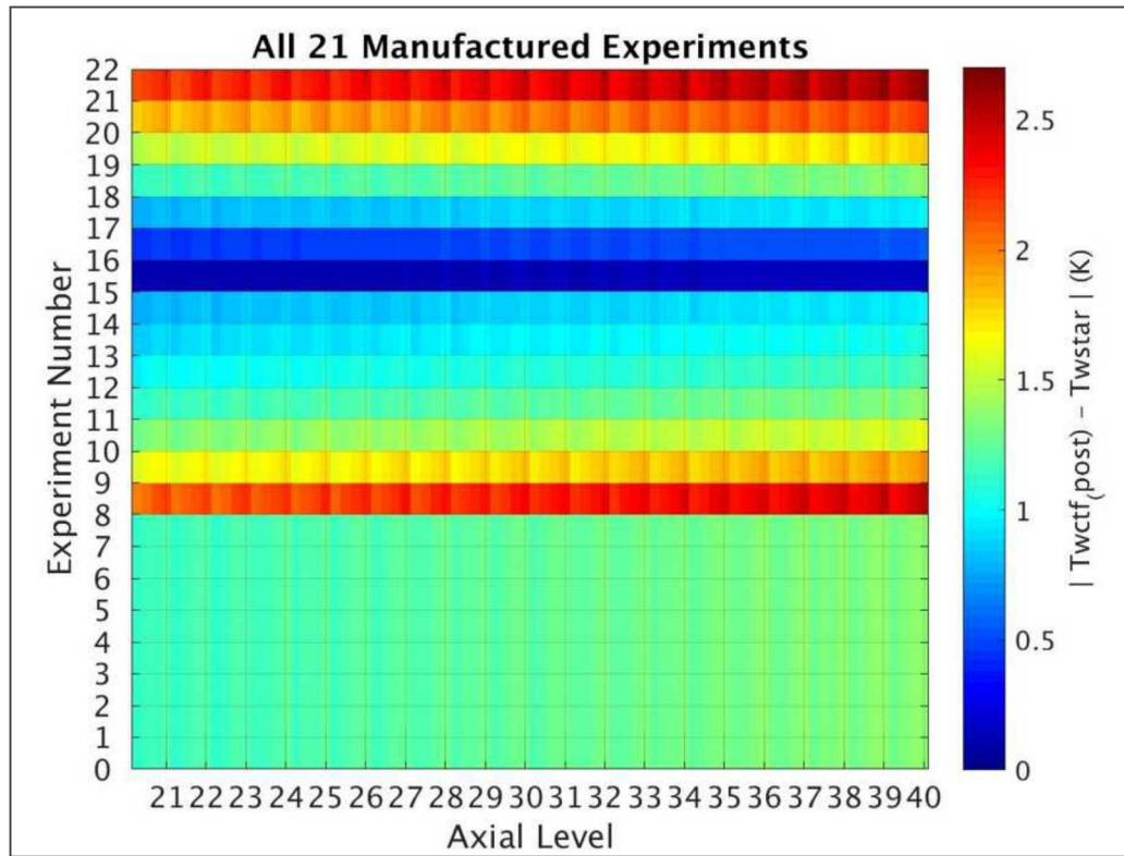
**Figure 15:**  $|\bar{T}_{w,CTF-post} - \bar{T}_{w,STAR}|$  plotted after calibration for 22 single channel datasets. Each row represents one of the 22 experimental tests in array form (every 4 columns represents 2 pi in  $\theta$  for each axial level).
