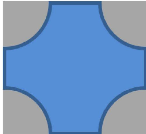
**Figure 13: STAR and CTF geometry for the single channel problem. The four quarter rods are treated as if they are one single rod and have the same applied heat flux.**
