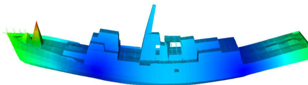
Figure 1: Wet Modes Calculation of a Ship
