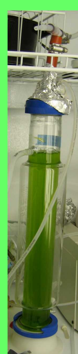
Fig 2. Airlift photobioreactor analysis to assess how photosynthetic adaptation to CO 2 affects lipid production. Low CO 2 levels in a culture induces carbon concentrating mechanisms (CCMs). It is unknown if investment in cellular machinery to run the CCM consumes lipid stores or if there is a net increase in storage from greater efficiency.
