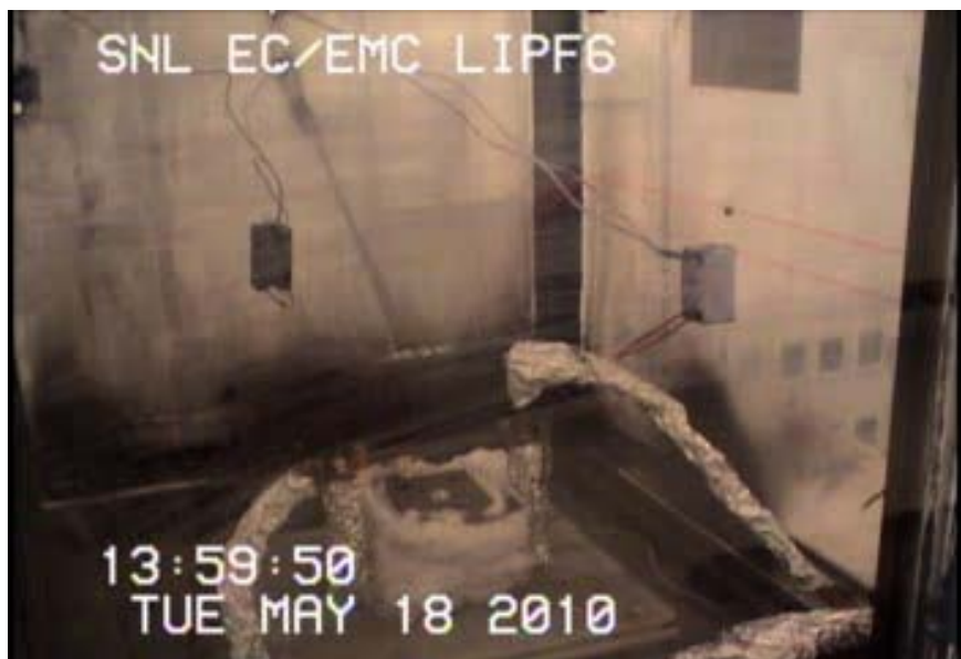
Ignition of EC:EMC electrolyte
