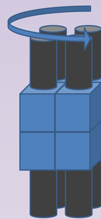
A disadvantage to the rotating mask is the fundamental concept that the mask must block source particles from reaching the detector, thereby lowering the source signal. This decreases the efficiency of the system and increases the count time to adequately locate the source.
