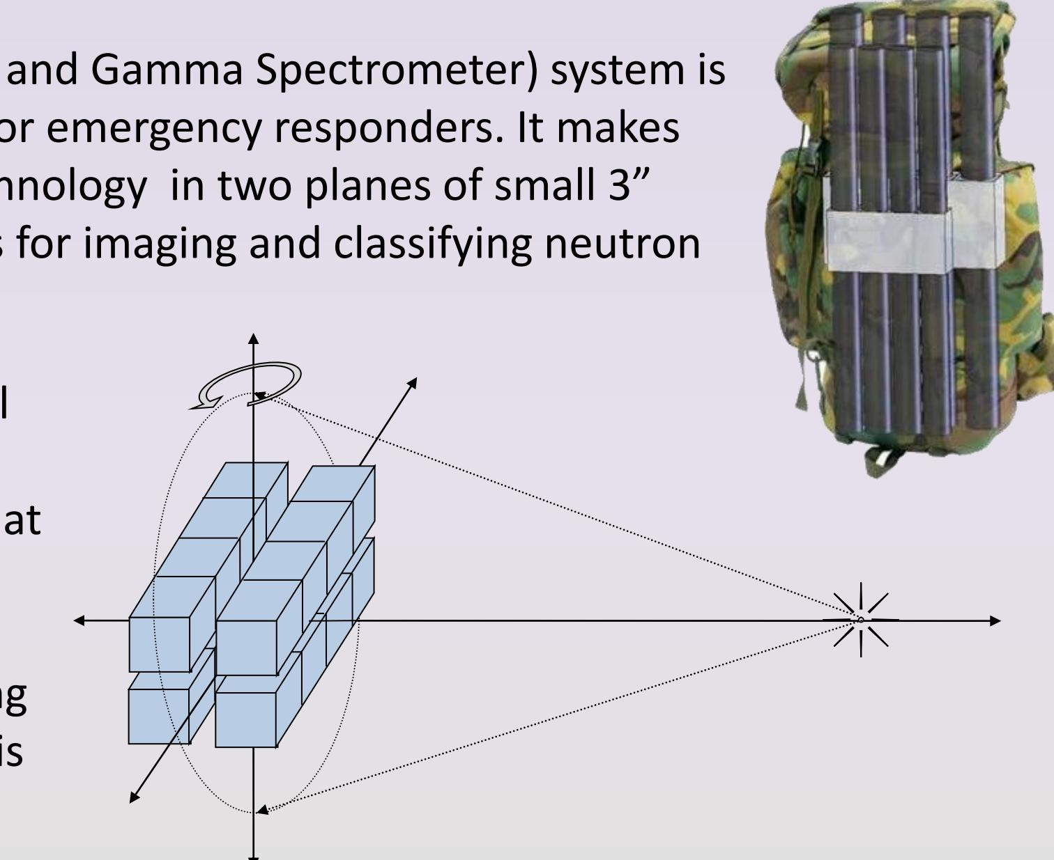
Rotating the detectors around a central axis to create a PRISM systems would allow for use of single scatter events that do not contribute to the NSC mode, increasing the efficiency greatly. In the case of emergency responders, reducing the necessary measurement time in this way is extremely advantageous.
