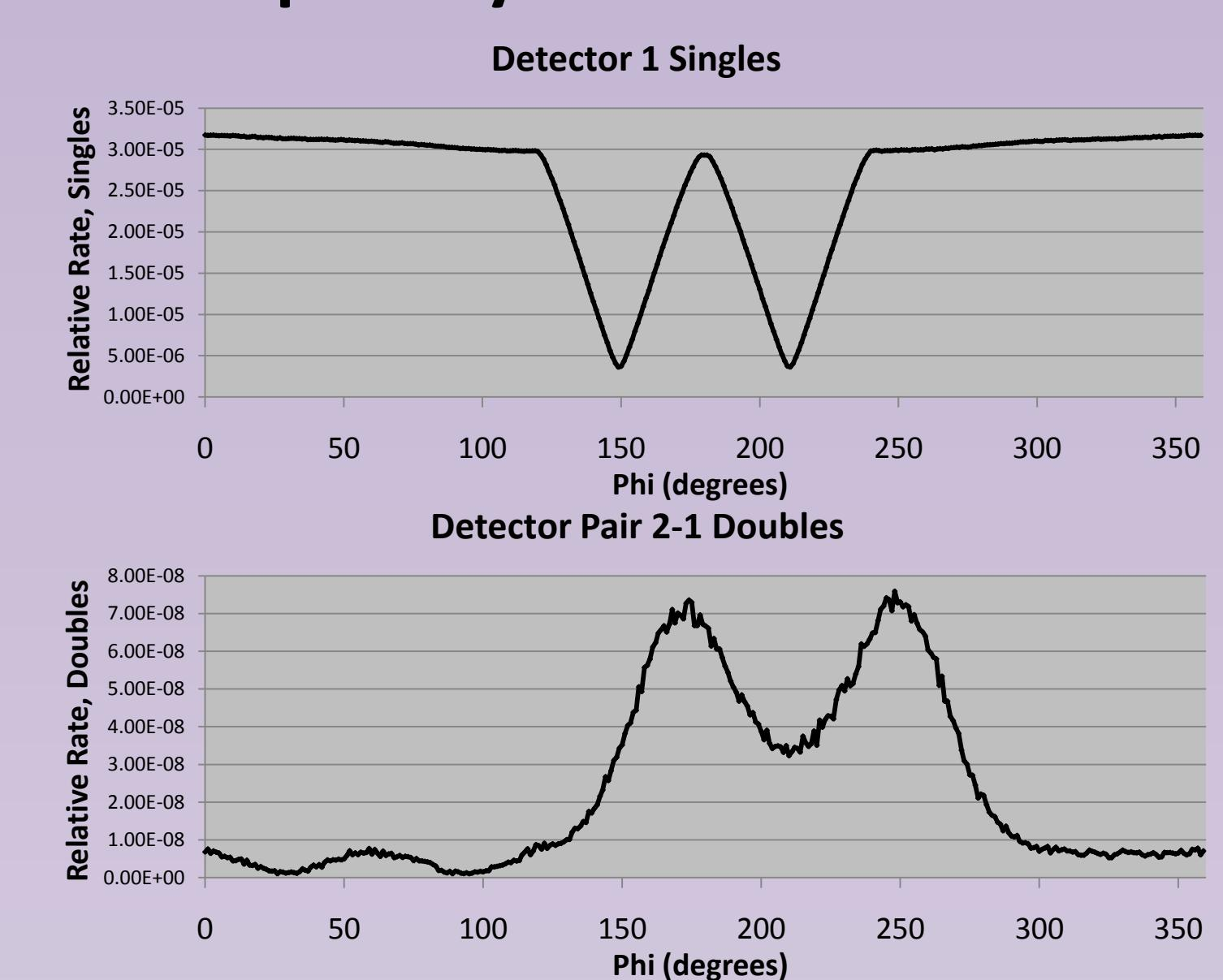
A stretch goal for the doubles mode is to incorporate the concepts of the Neutron Scatter Camera (NSC). The NSC is a proven system that uses neutron double scatters between two detector planes to find the direction of the incoming neutron. With many interactions, the source location can be identified with great accuracy. PRISM could be configured to record the positions of each detector pair during a double scatter to calculate this direction for an added precision.
