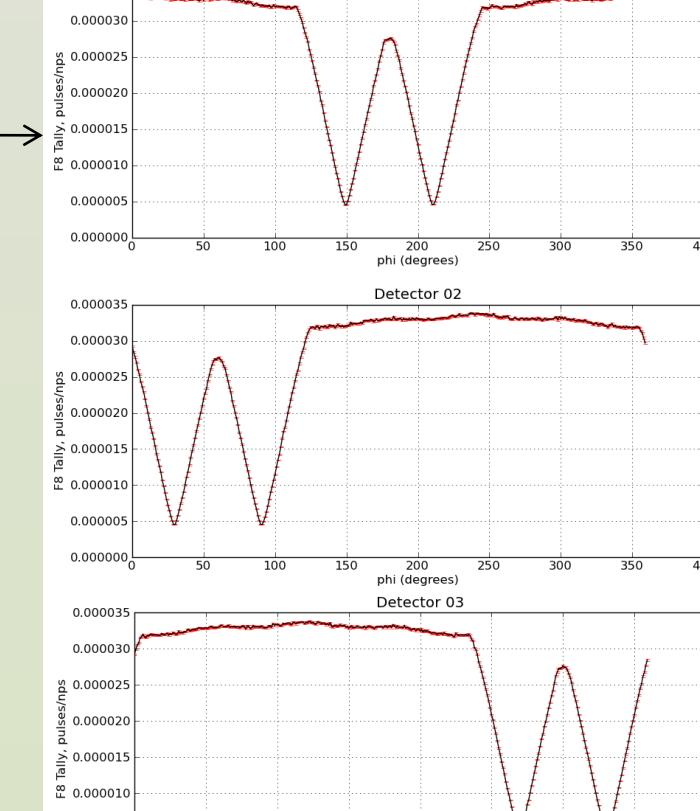
The Python script loads a geometry template file, writes and executes an MCNP input file at each rotation angle, and extracts the resulting performance data. It returns a response function, shown right, for each detector.
