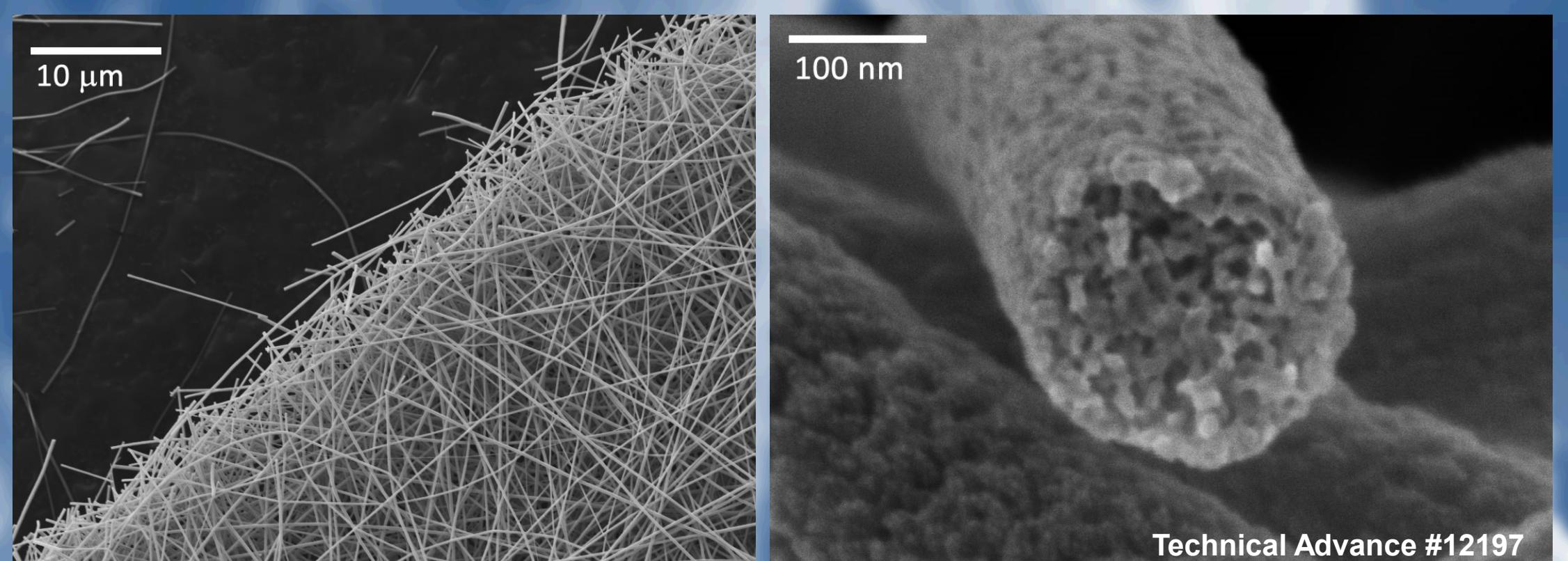
Scanning electron microscopy (SEM) images of the TiO<sub>2</sub> nanofibers show the typical achievable porosities: (a) inter-fiber microporosity, (b) intra-fiber nanoporosity.
