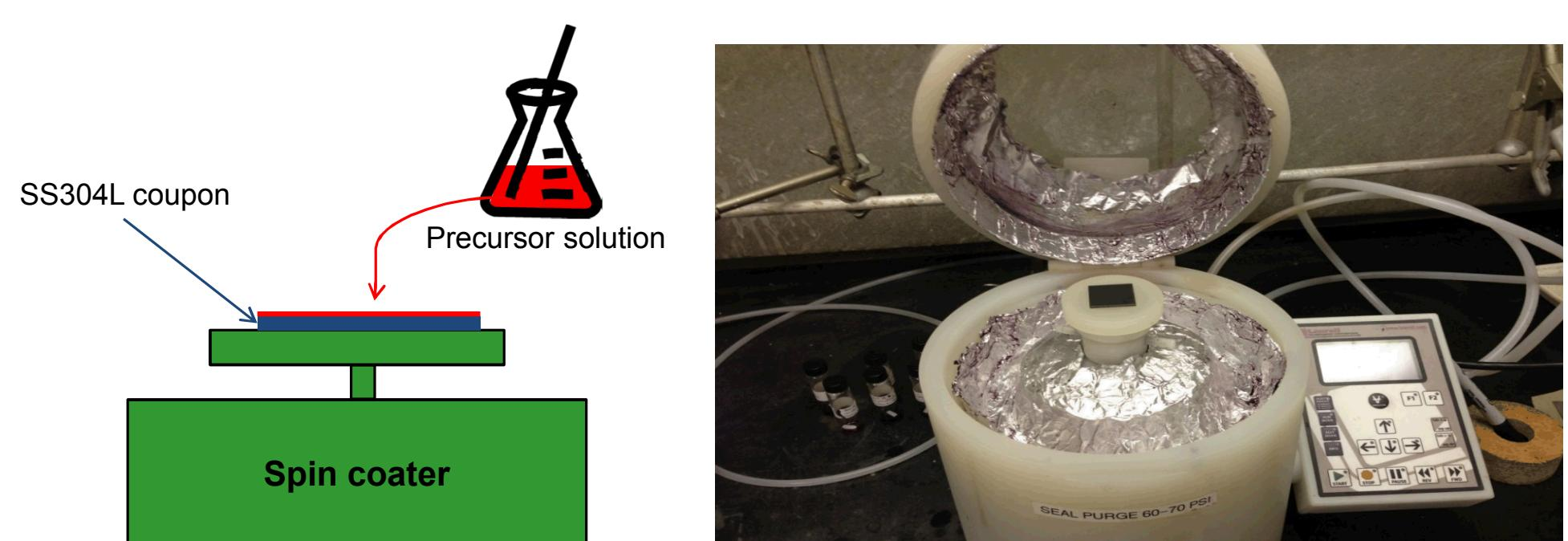
The spin coater is used to produce a thin layer of solution with each spin. The stainless steel coupon is held to the spinning shaft using a vacuum pump.
