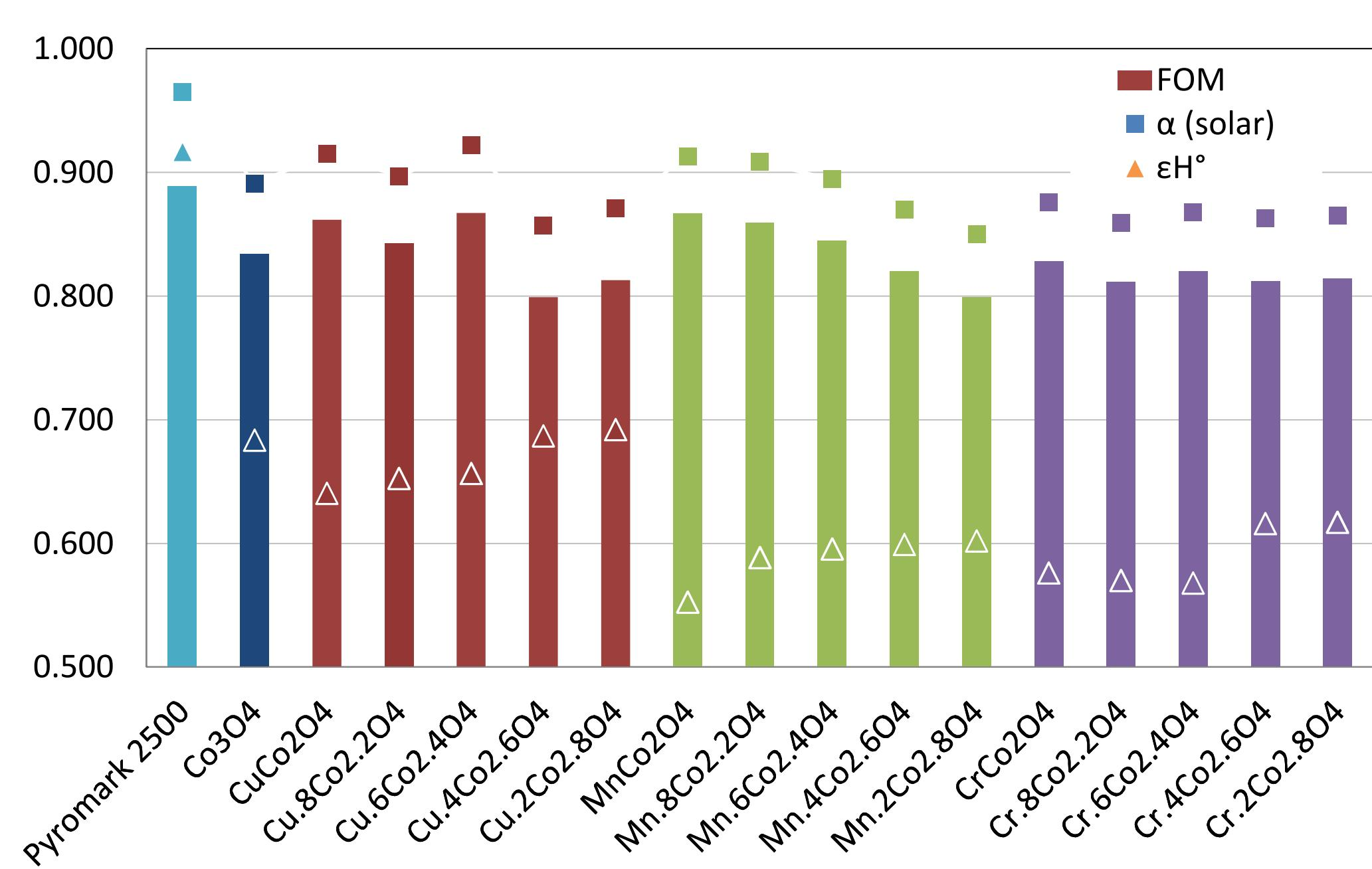
The absorptivity, emissivity and figure of merit for each of the materials are shown here. Absorptivity is indicated by the square, emissivity is shown by the triangle, the figure of merit is designated by the bar. Each different Transition metal series is the same color.
