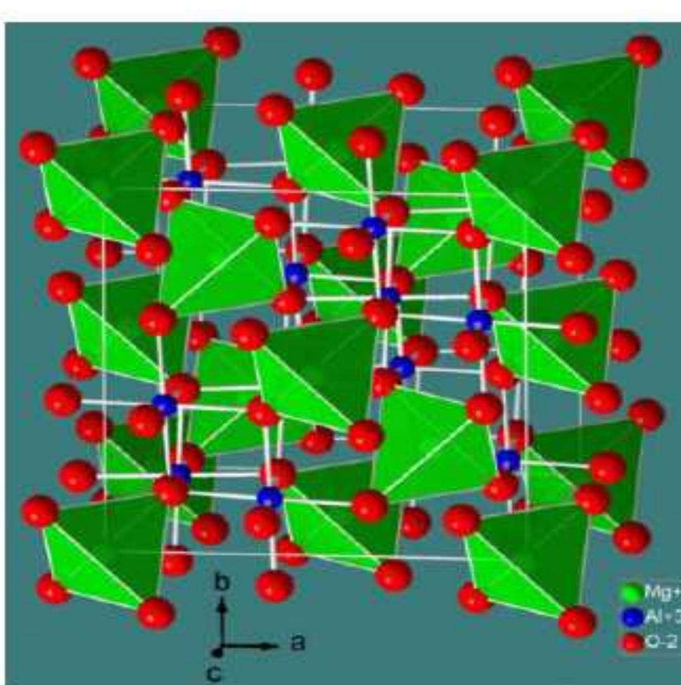
Metal oxide spinels with the composition  $\text{AB}_2\text{O}_4$  were chosen as target materials for solution-based deposition methods because of their inherent high temperature and oxidation stability. Cobalt-based metal oxides ( $\text{Co}_3\text{O}_4$ ) have shown promise as selective absorber materials and were chosen as a base for this study.
