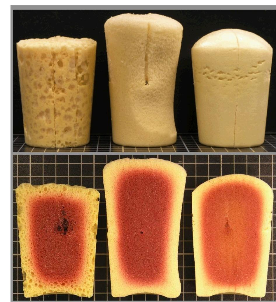
Uniform changes in color observed with aging at elevated temperatures.
