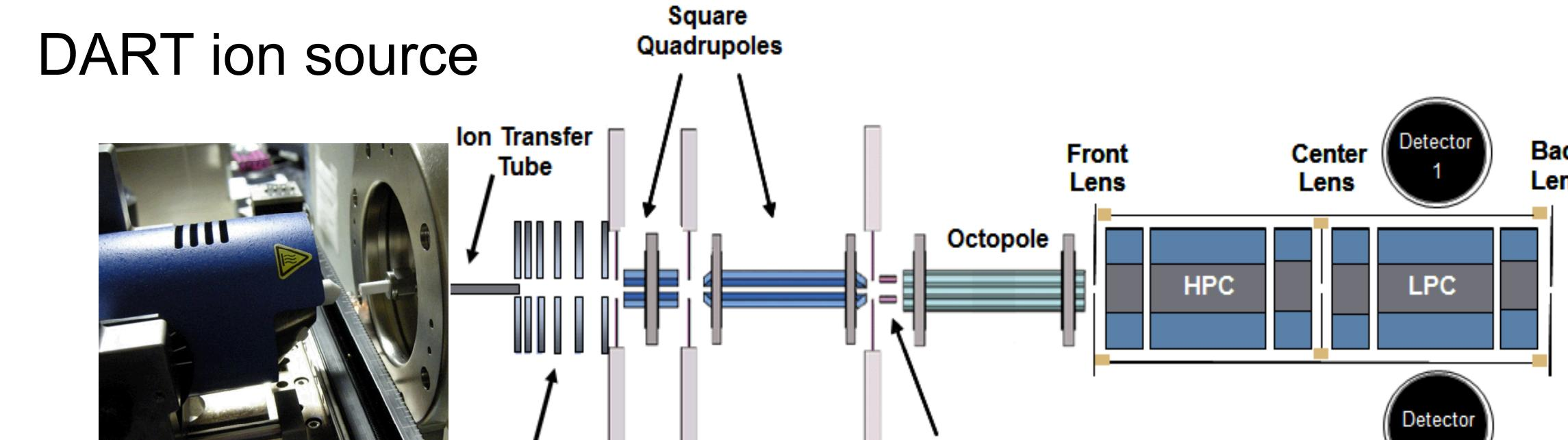
MS<sup>n</sup> with Ion Trap Mass Spectrometer.
