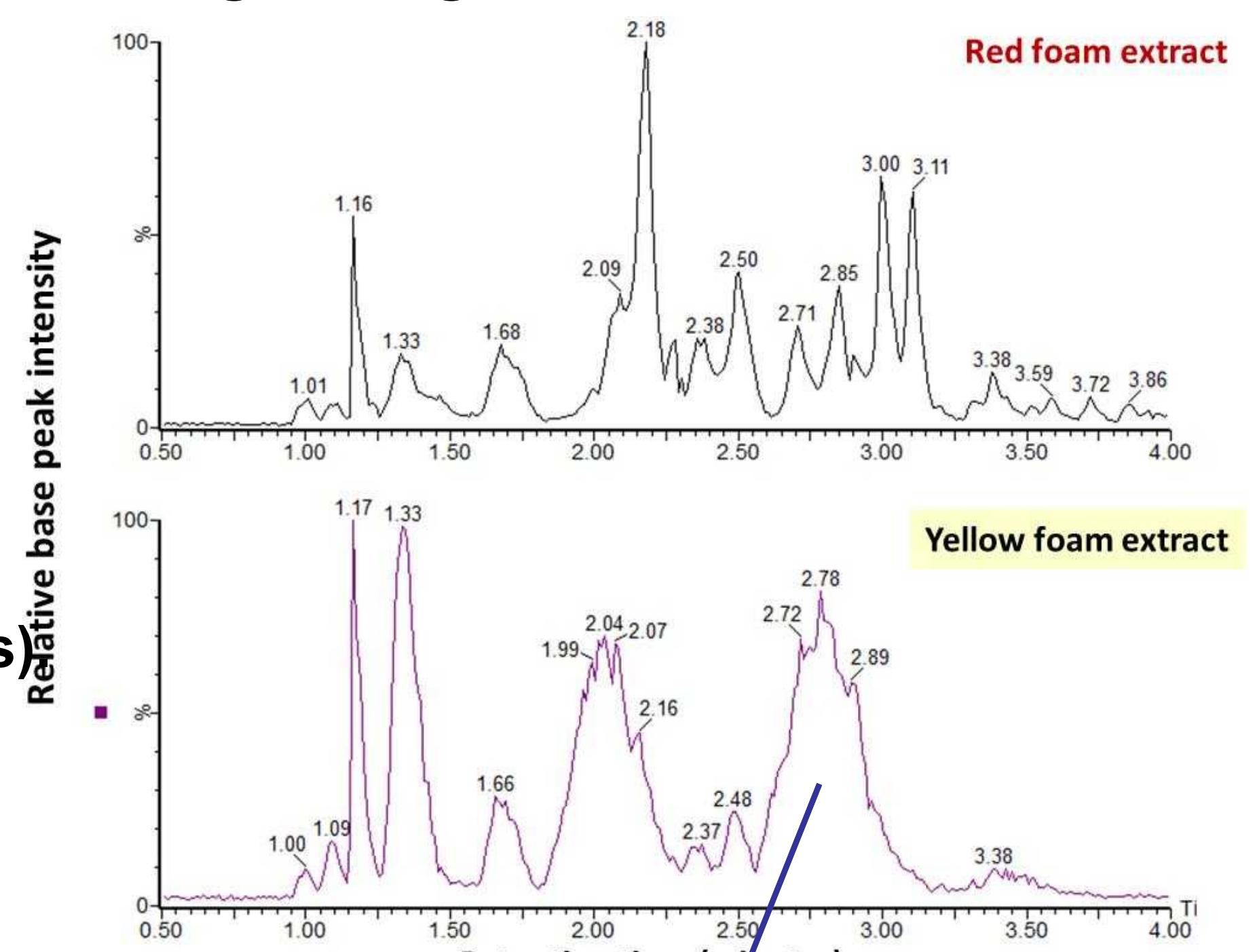
Among the differences observed – a m/z 592 with 8x higher intensity in red versus yellow foam. DART/MS with MS<sup>n</sup> is underway to determine the chemical identity. This m/z is not a precursor or known reactant.
