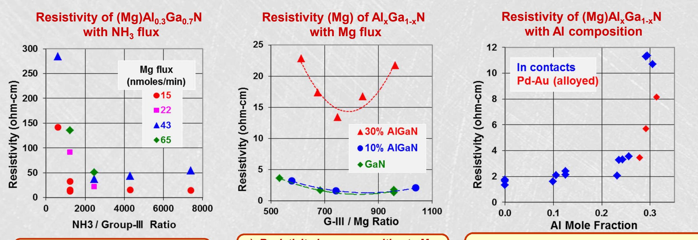
Mg-doped  $\text{Al}_x\text{Ga}_{1-x}\text{N}$  test structure
