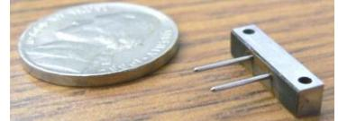
*Plug-and-Play optical array contains twelve laser and photo-diodes.*
