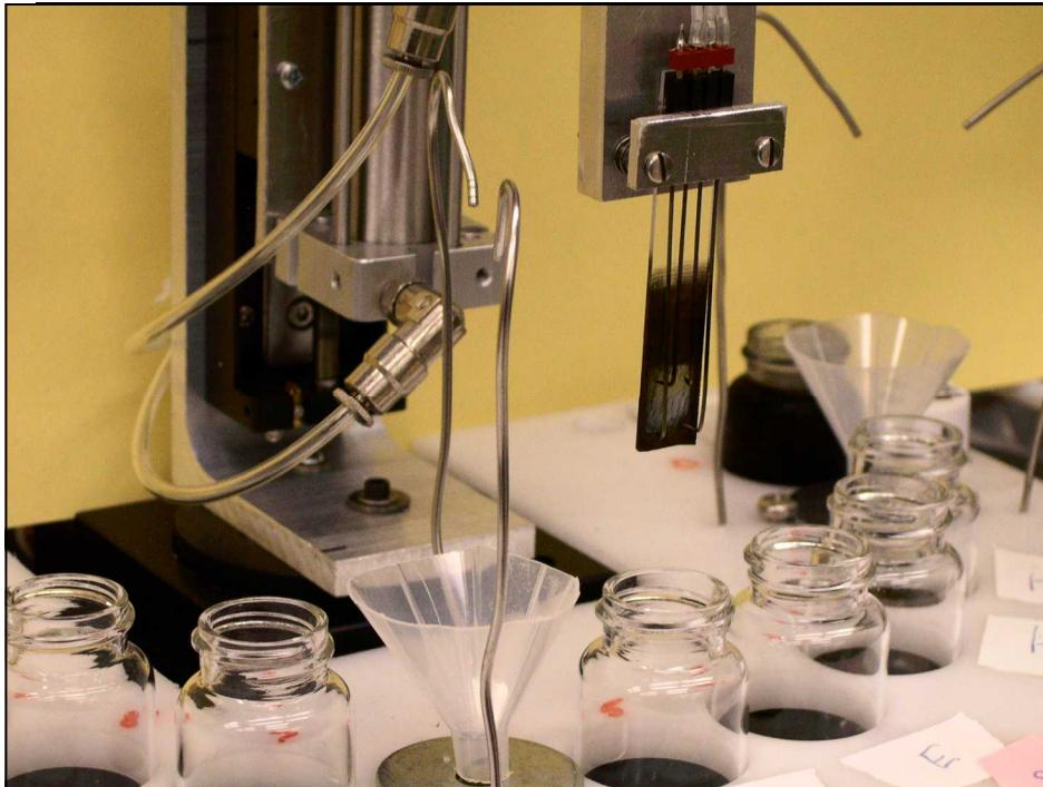
Through a series of steps the robot iteratively assembles nanoparticle – ligand layers creating a conducting film.
