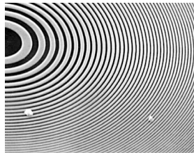
X-ray "lens" ring spacing \sim 35 \text{ nm}
