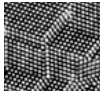
Atoms of silicon spacing ~ 0.2 nm
