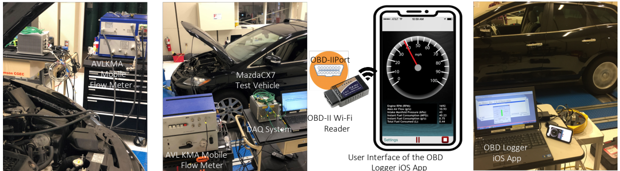
Figure 47: The AVL KMA Mobile fuel measurement system and the OBD-based fuel rate estimator connected to the combustion test vehicle
