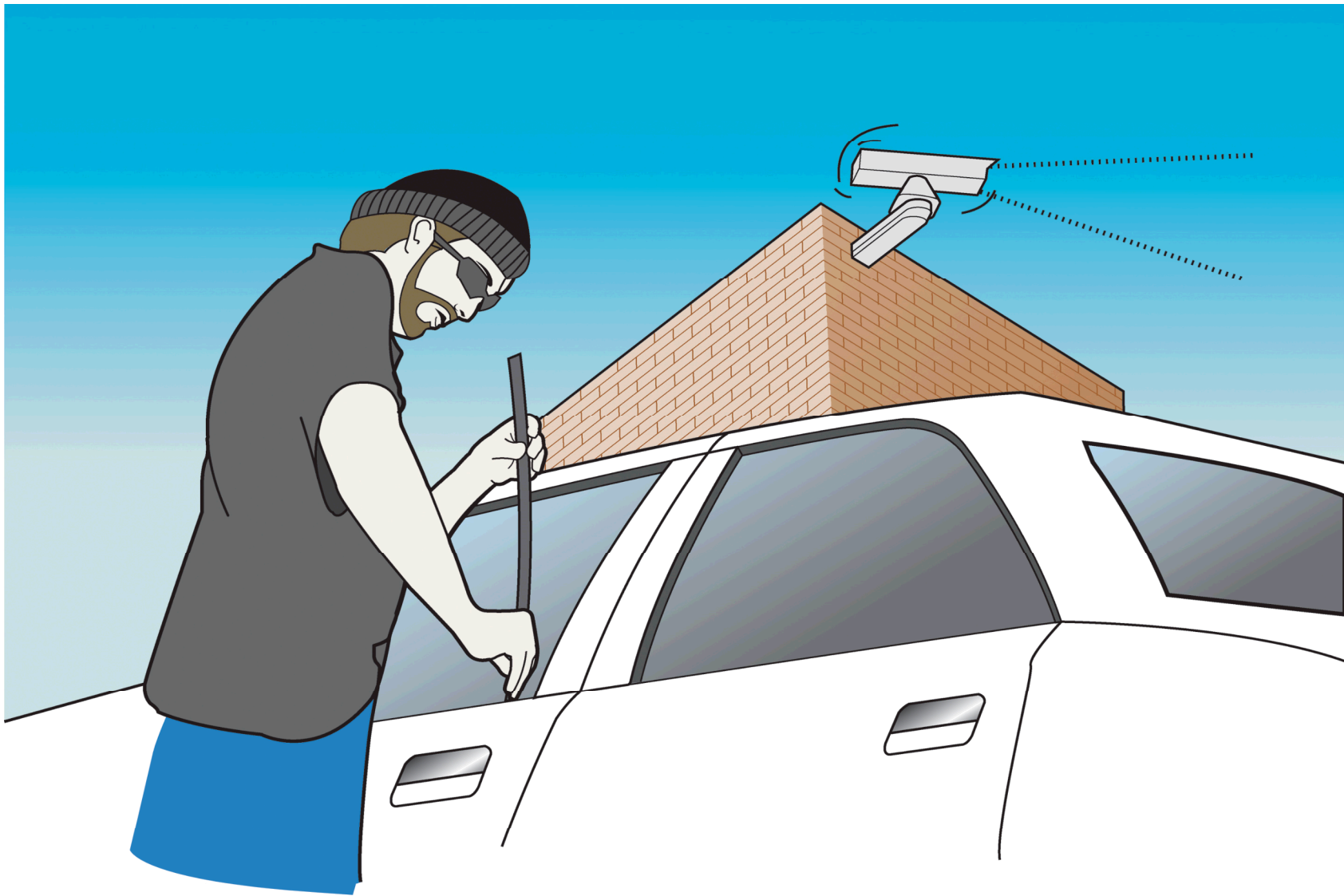
Figure 7.2 A pan-tilt-zoom camera that is set to automatically pan an area may completely miss capturing incidents of concern.
