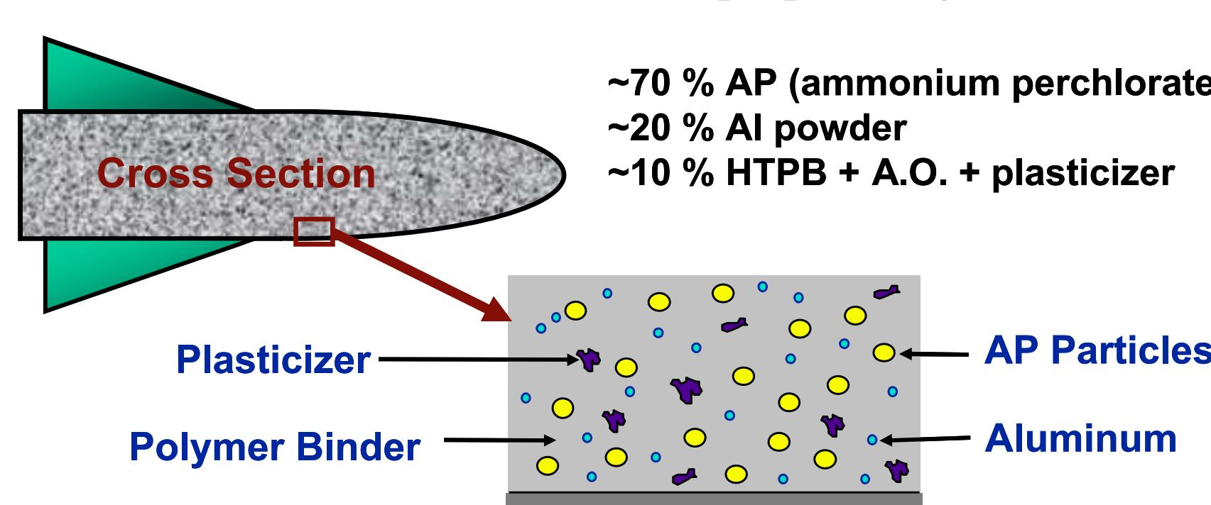
Of the various components in the composite propellant, the HTPB binder ages most rapidly, thus affecting the overall propellant performance.
