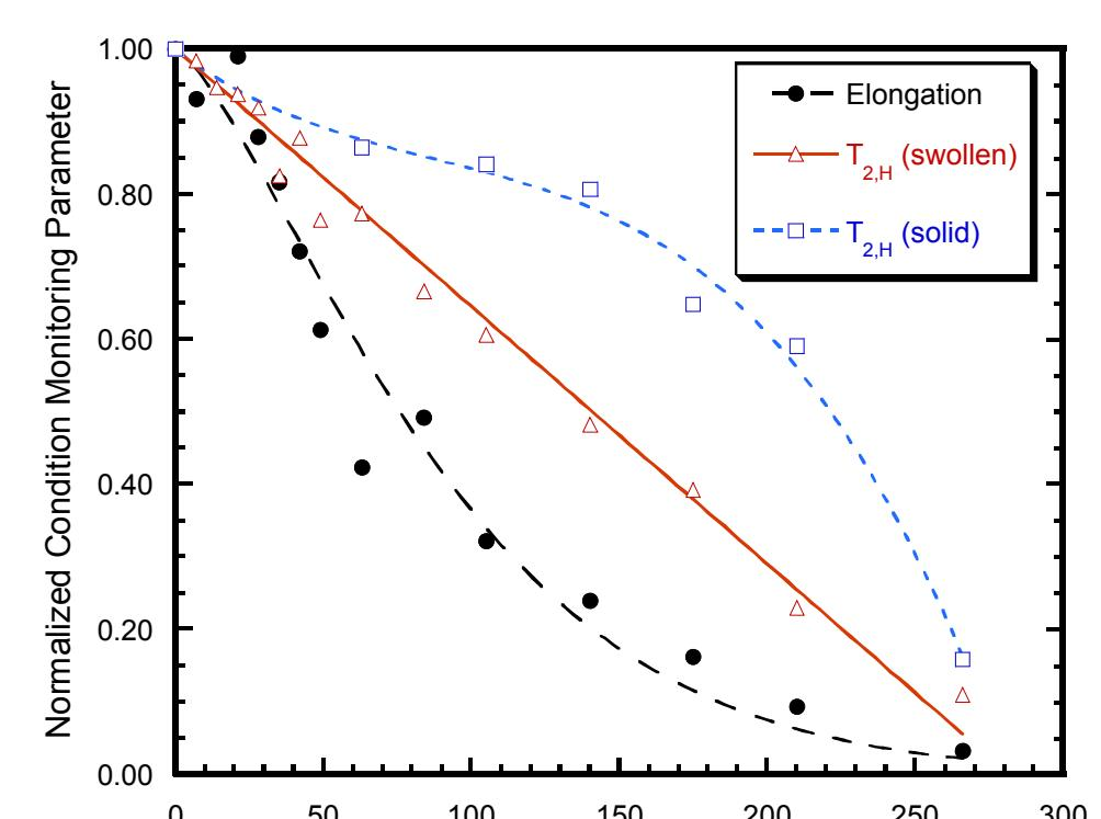
$^1\text{H}$   $T_2$  relaxation times of solvent-swollen HTPB samples are **more sensitive** to thermo-oxidative aging than  $^1\text{H}$   $T_2$  times of solid HTPB samples.
