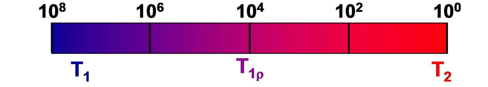
Different relaxation times can probe a wide range of molecular motion rates which may reflect different molecular processes.
