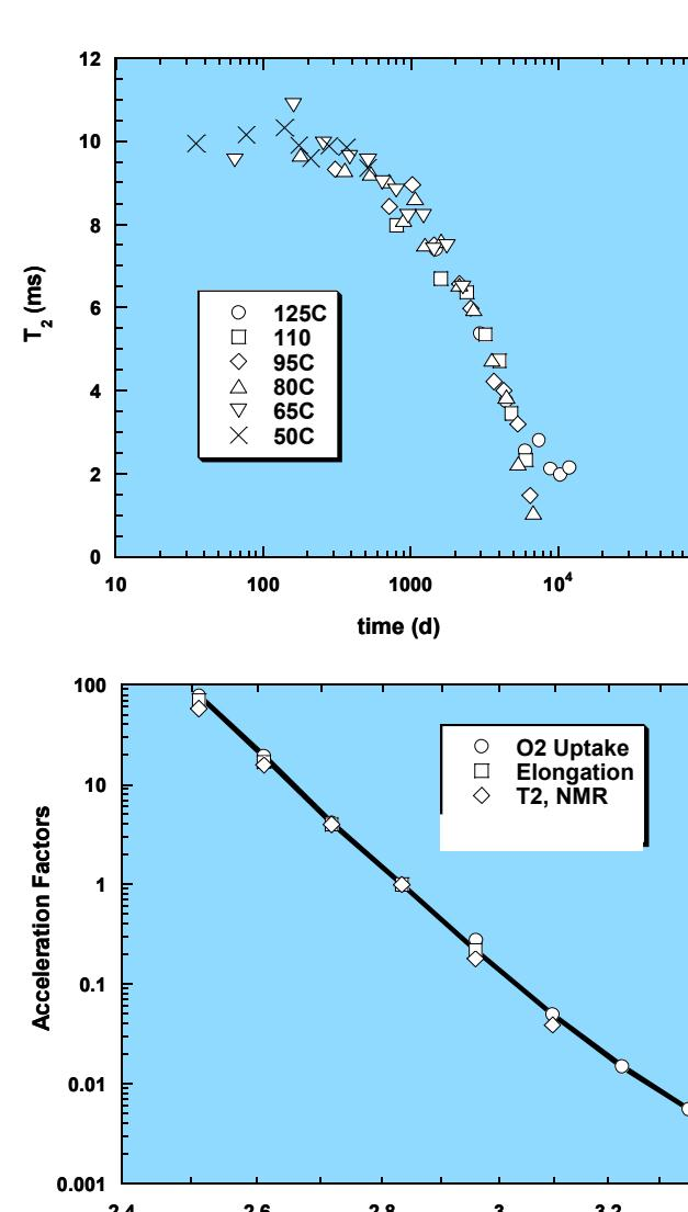
The acceleration factors for  $^1\text{H}$  NMR  $T_2$  of swollen HTPB agree with those derived from elongation and oxygen consumption measurements.
