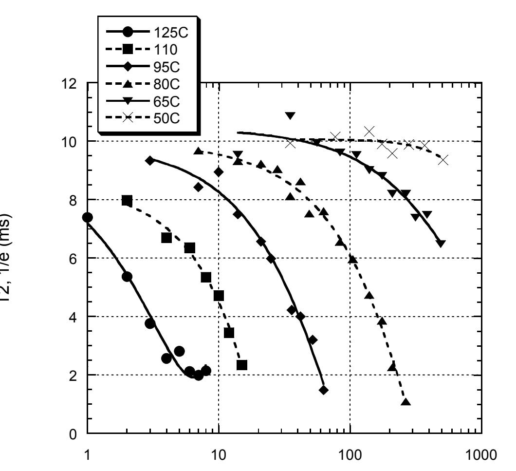
The higher temperatures (110 and 125 °C) exhibit diffusion limited oxidation.
