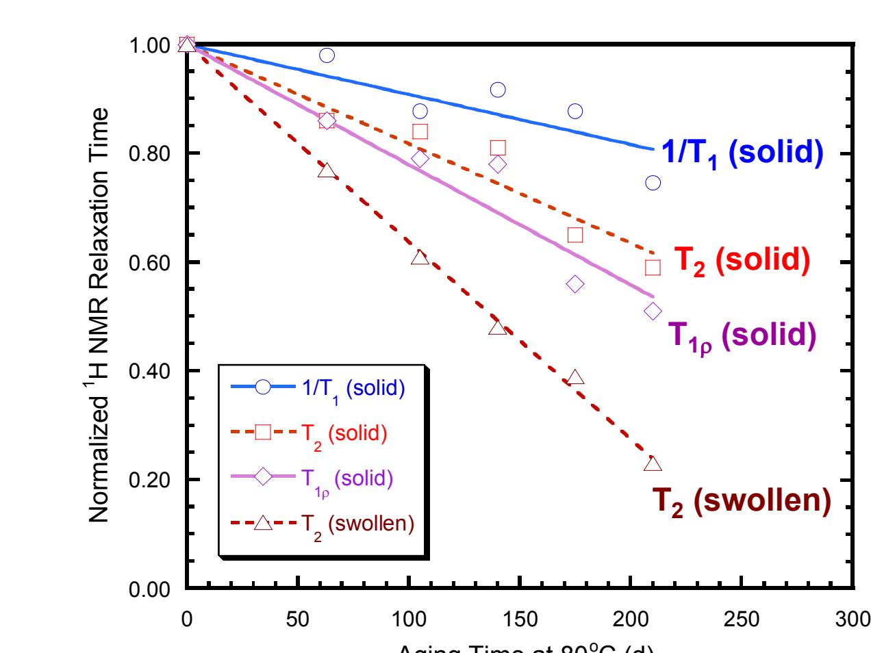
Sensitivity:  $T_2(\text{swollen}) > T_{1p}(\text{solid}) > T_2(\text{solid}) > T_1(\text{solid})$
