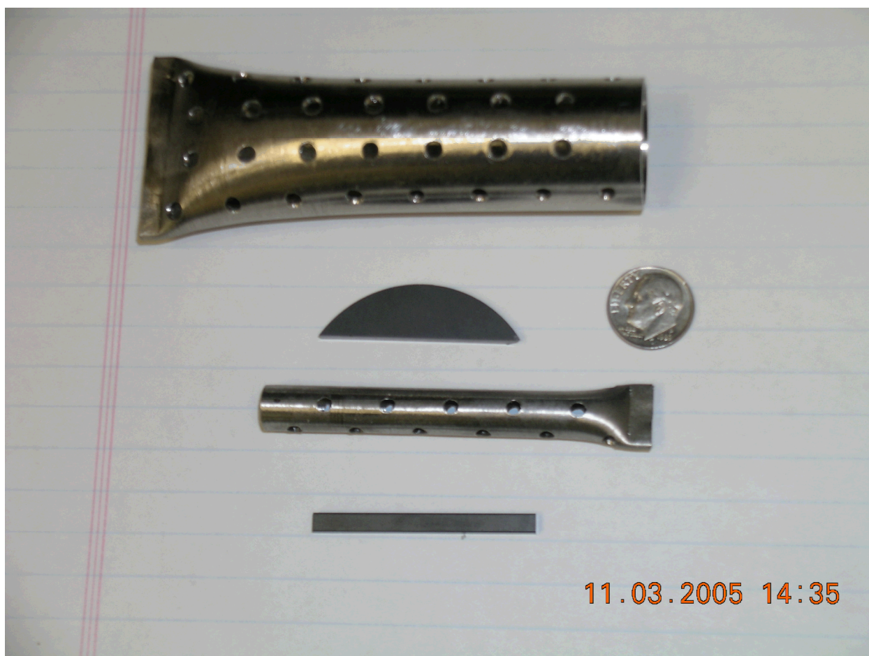
Figure 9. Perforated Hastelloy tubes used to hold samples for corrosion testing. The larger diameter tube was placed at the bottom of the boiler, and the smaller diameter tubes were placed below the catalyst bed. The samples shown are pieces of silicon carbide.
