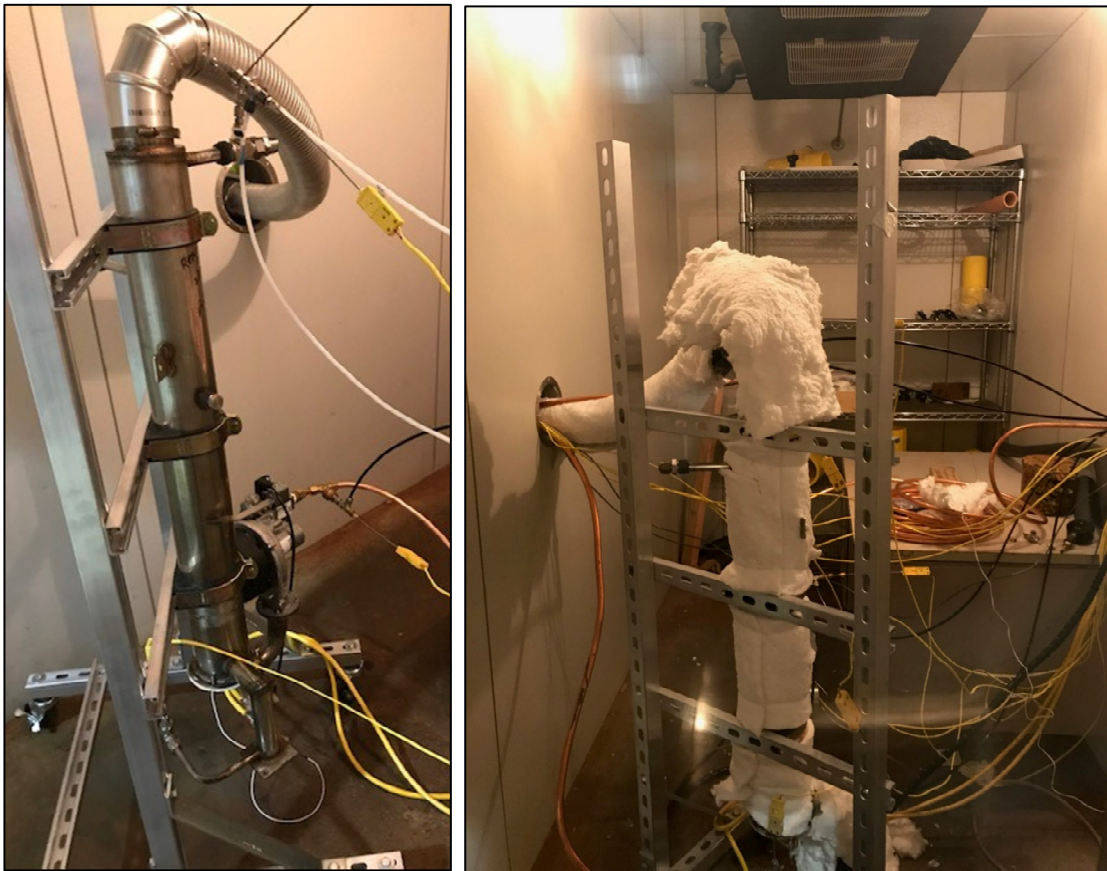
Figure A6: Uninsulated (Left) and Insulated (Right) Test Setup within Chamber
