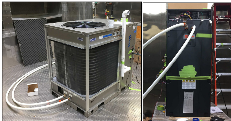
Figure 3: GAHP installed in ‘outdoor’ test room (left), AHU installed in ‘indoor’ test room (right)
