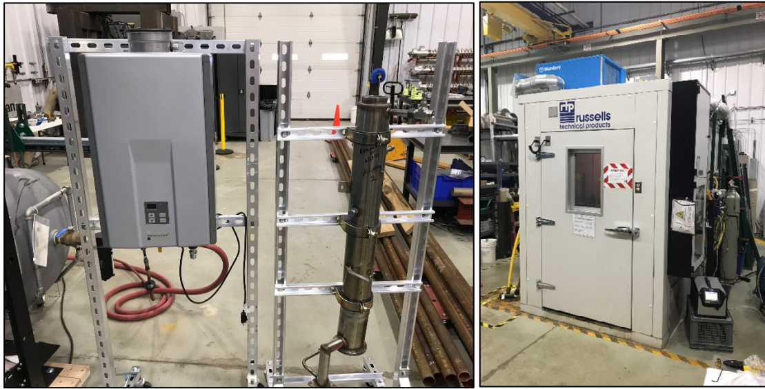
Figure A4: “Dummy Desorber” with pre-heating tankless Water Heater (Left), Cold Climate Chamber (Right)
