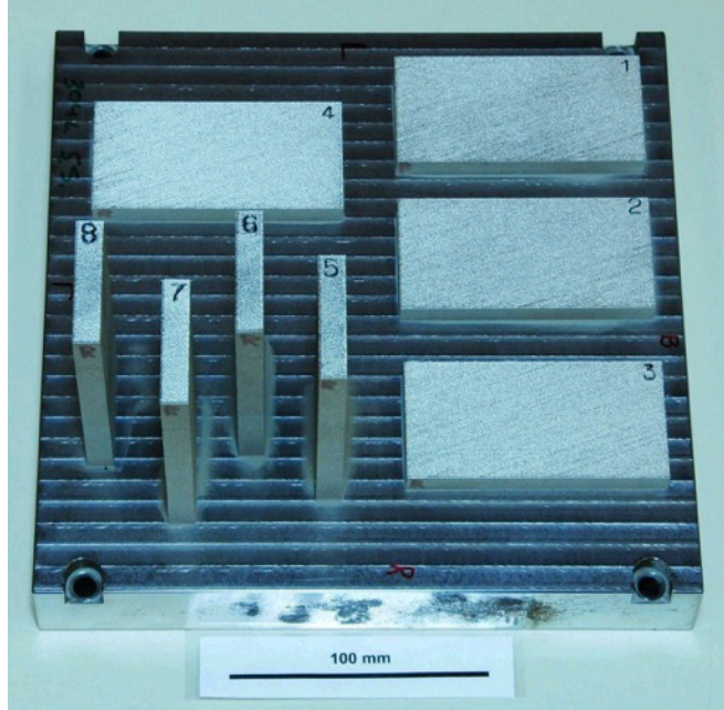
FIG. 1. Optical photograph of EOS builds on 304L stainless steel baseplate.
