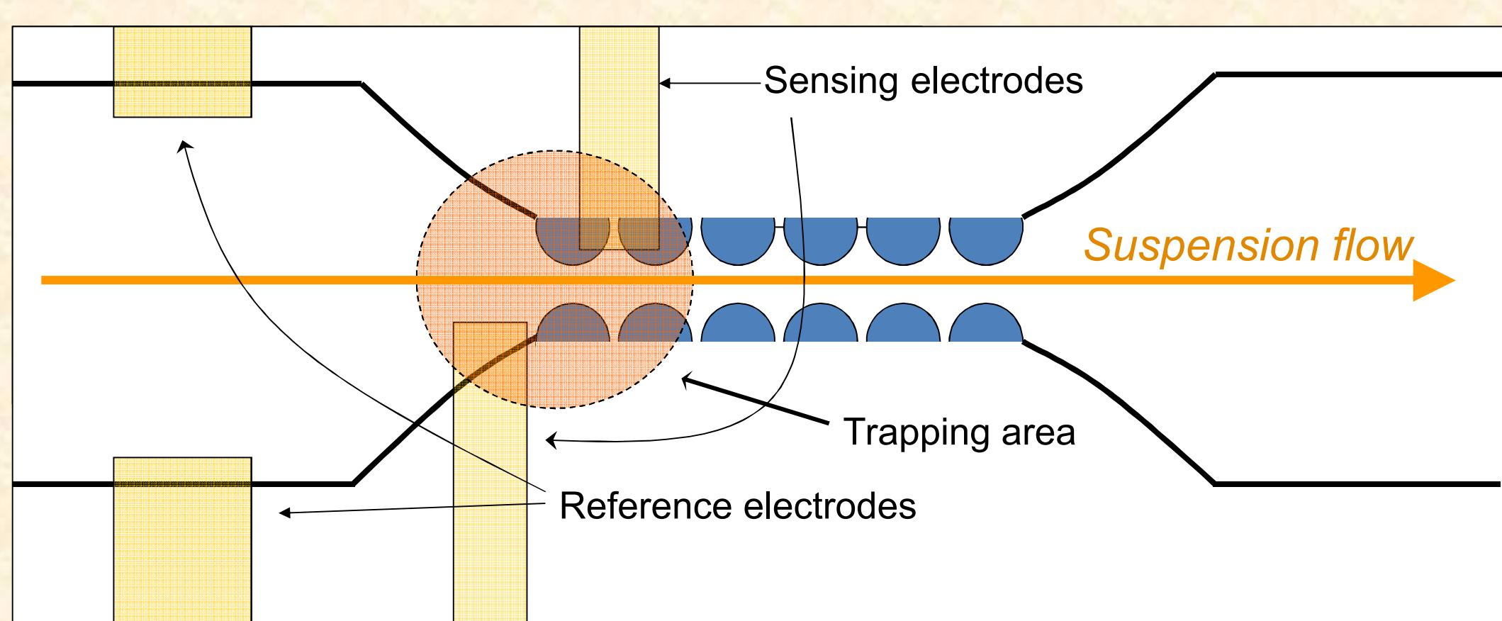
**Electrodes in the detection area are passivated with  $\text{SiO}_2$  to prevent air bubble formation in the fluid samples.**
