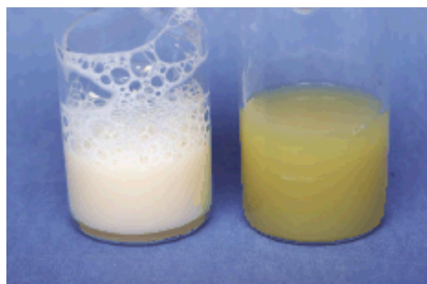
Figure 4. Digital image of a dye-containing emulsion with 20 mM of the carboxylate Diels-Alder DA surfactant before and after exposure to 95 °C for 2h.
