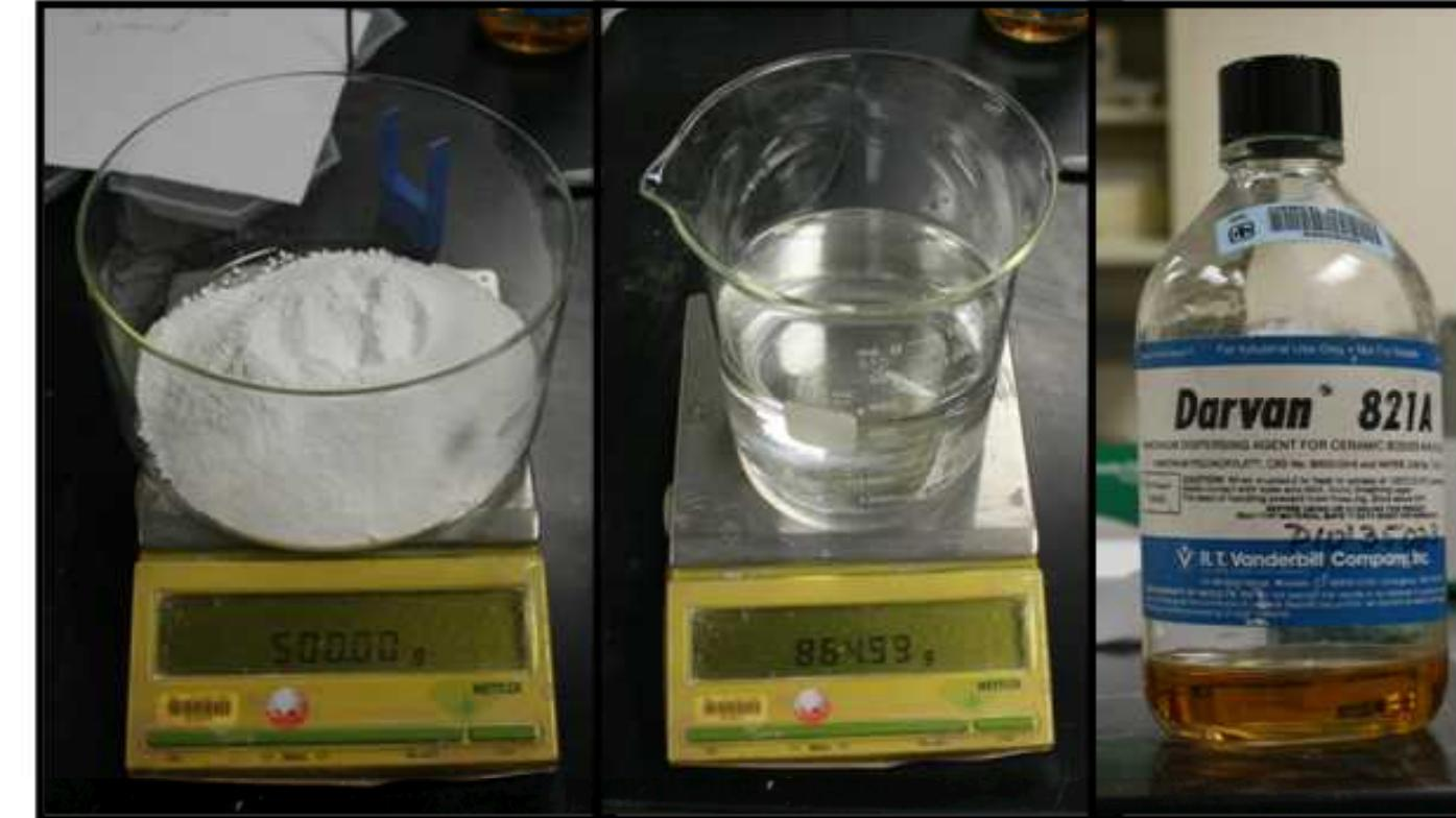
The 0.2  $\mu\text{m}$  ZnO powder is weighed out and mixed with DI water and a dispersant.
