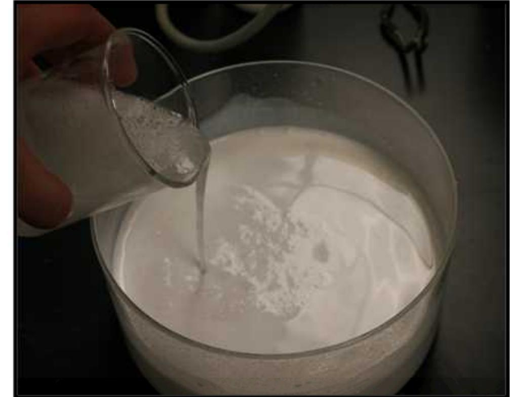
A 3 wt% PVA/PEG binder is added to the slurry followed by ultrasonication.
