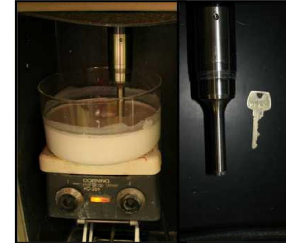
The slurry is ultrasonicated to break the agglomerates into individual particles.
