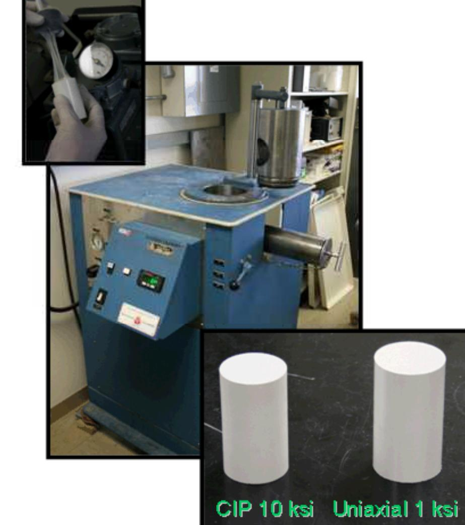
Each of the identically uniaxially pressed slugs are vacuum sealed and CIPed to incremental densities.
