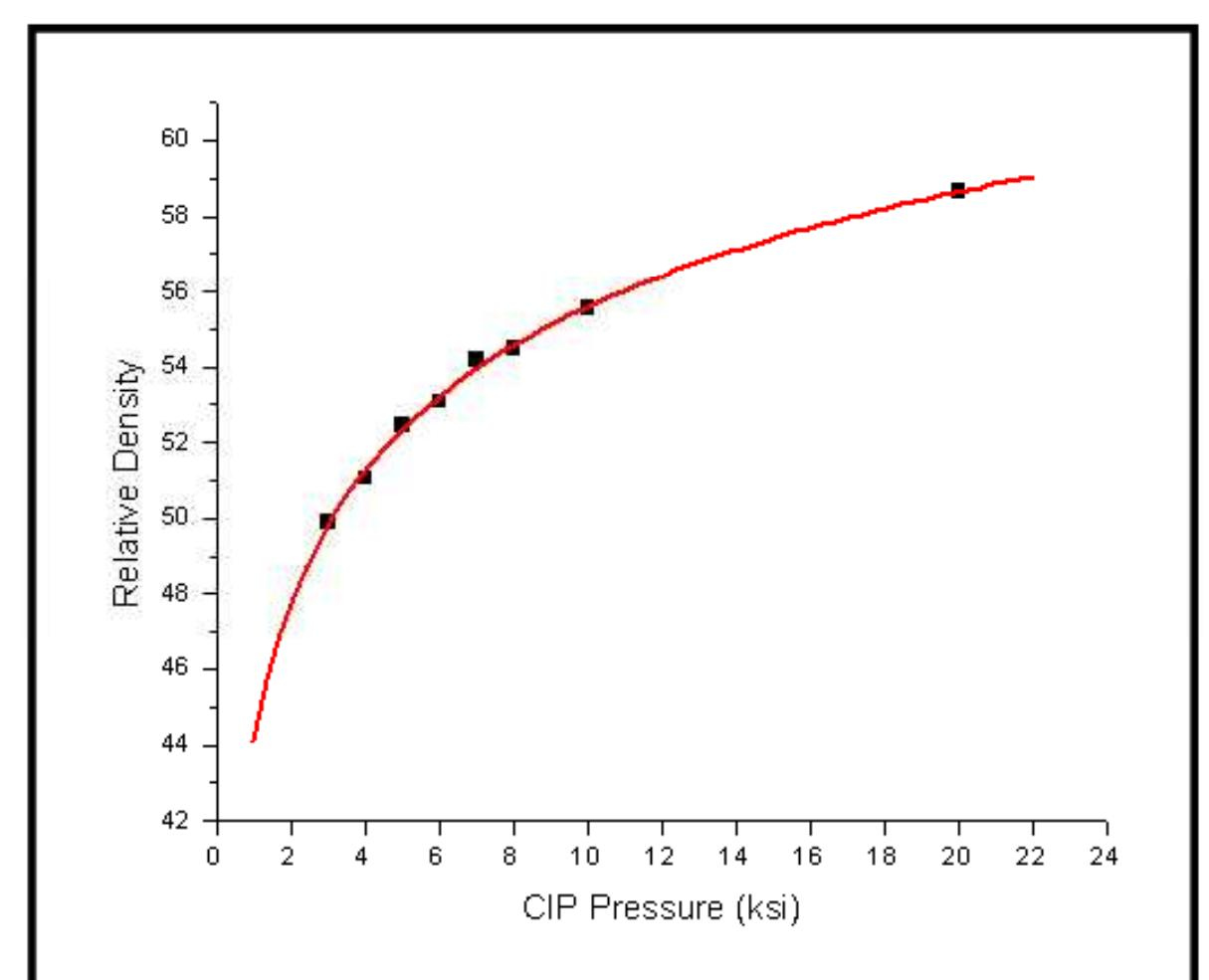
This plot shows the effect of CIP pressure on relative density. The large smooth asymptotic density change from pre-formed to 10 ksi CIPed is typical of a high-quality pressing powder.
