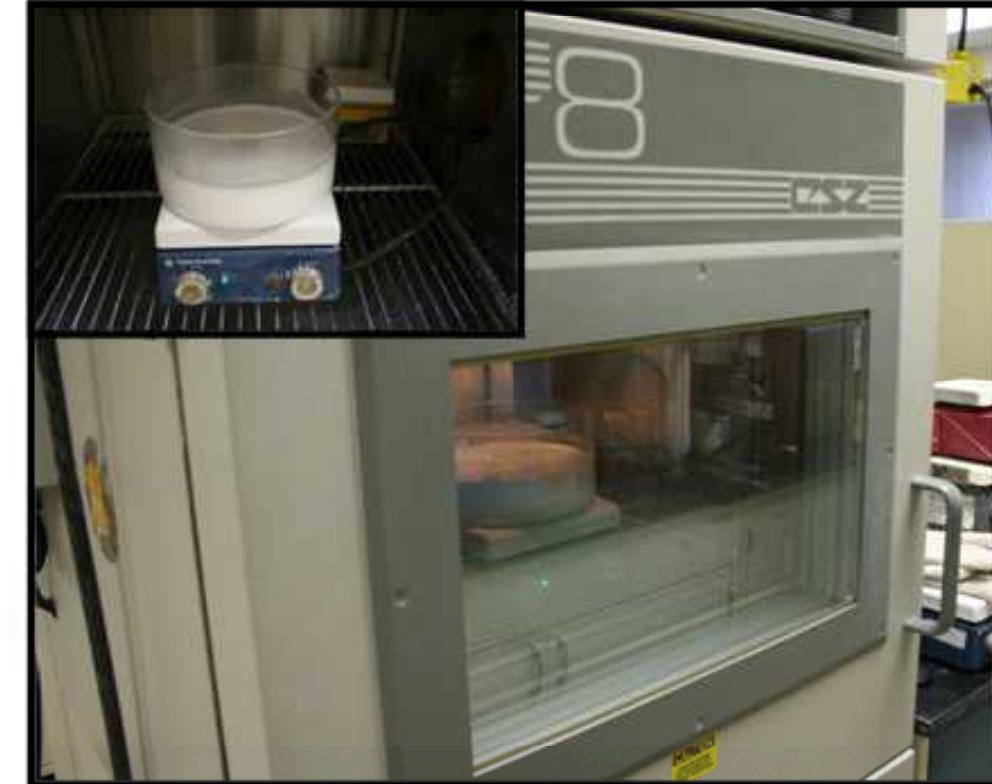
The water is driven off in a drying furnace at 70°C.
