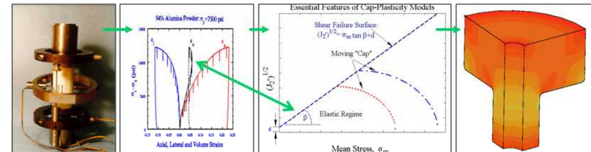
Tri-axial testing generates a plot of axial, radial, and volumetric strain of the powder compact. The inflection point on the volumetric strain curve reveals the stress state that corresponds to the shift from the elastic to plastic regime and defines the shear failure surface. When combined with the "cap" stress, it is used to model density as a function of stress state within finite element compaction models.
