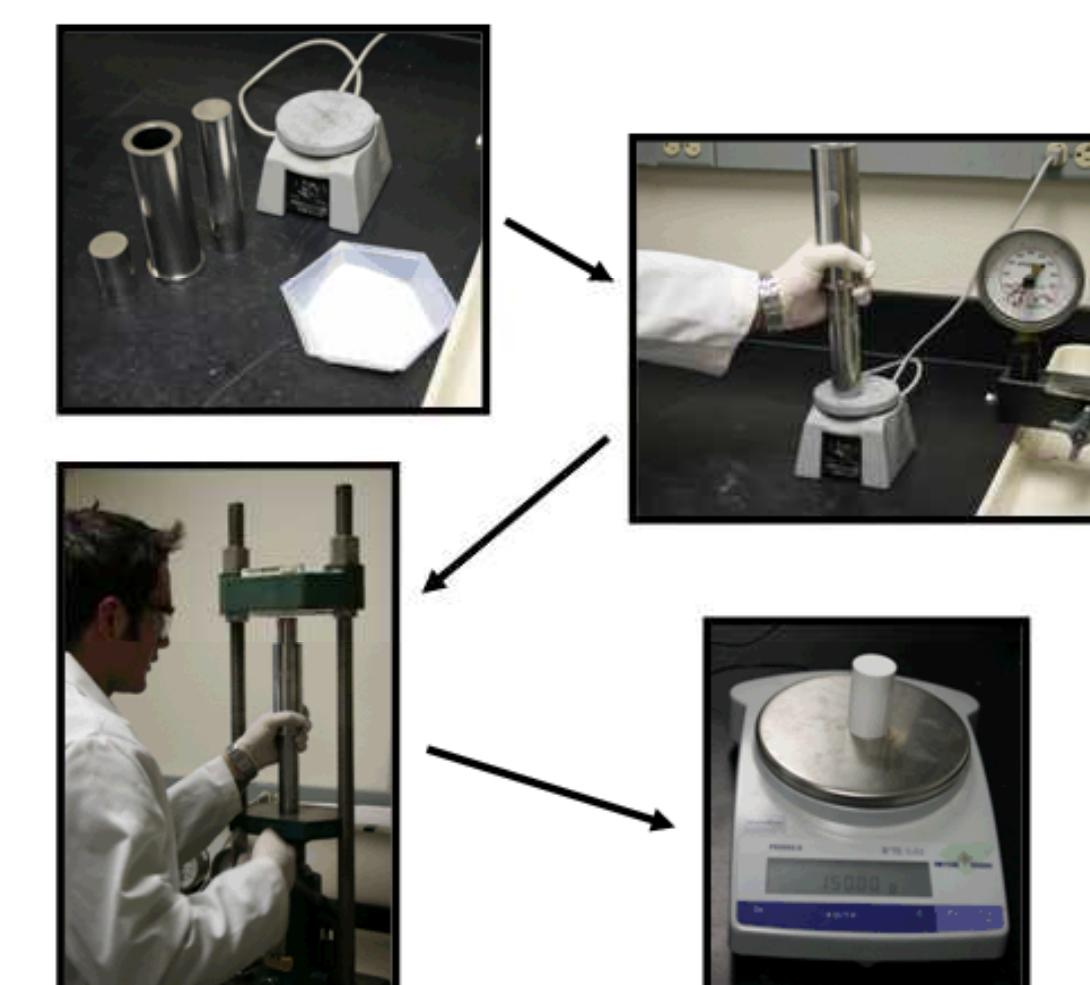
Powder is precisely weighed out, vibration packed, and uniaxially pressed into slugs.
