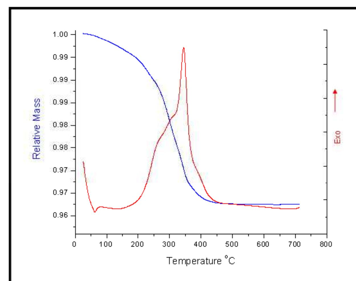
The thermogravimetric and differential thermal analysis plot shows the uniform binder burnout characteristics of the granulated powder.
