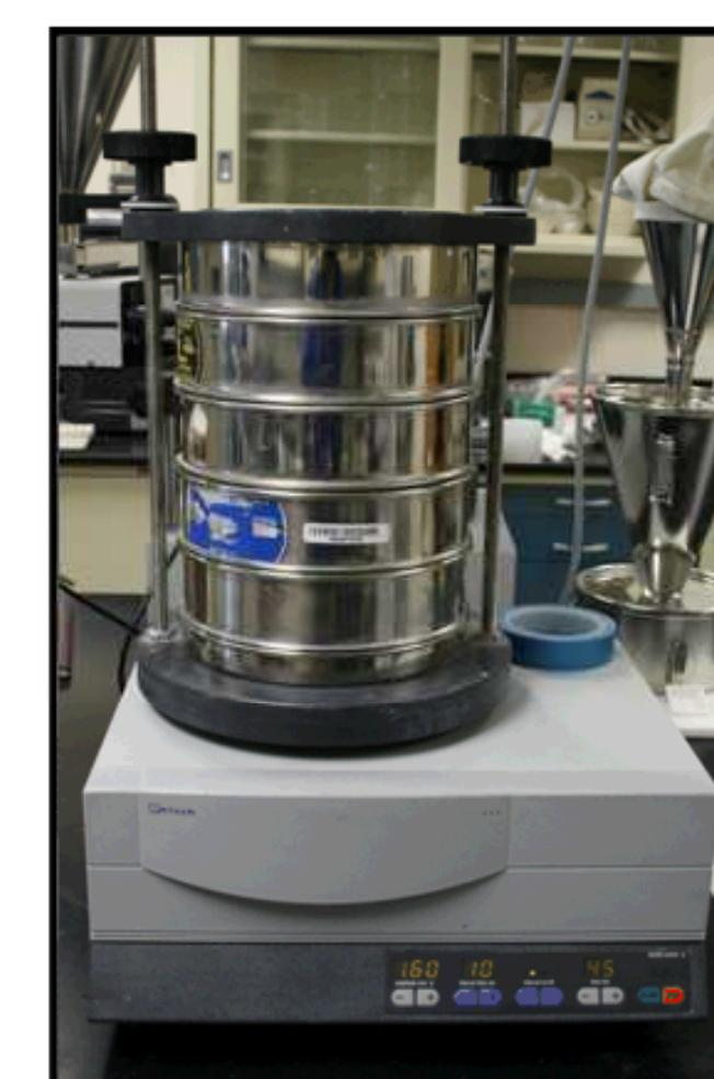
The granules are separated according to size with sieves. Large granules flow easily. Small granules tend to cake.
