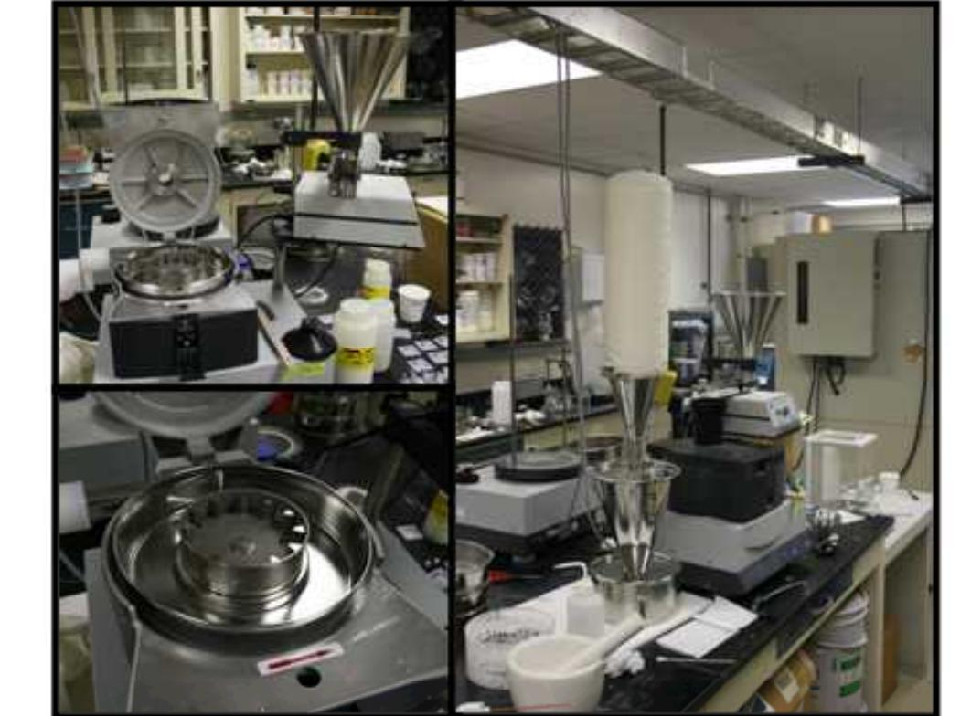
The dried powder is granulated in a high speed impact mill.
