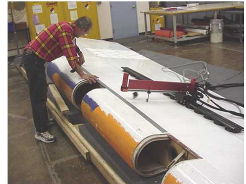
Developed P-E UT inspection – added for carbon laminate lug
