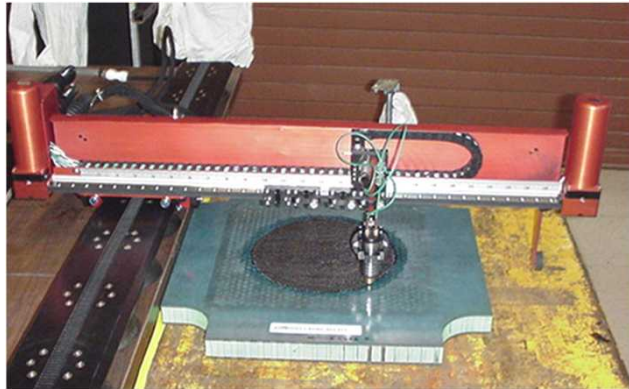
MAUS Inspections of Repaired Composite Sandwich Structures
