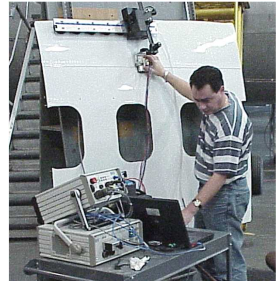
RD Tech Performing Blind Corrosion Detection Study
