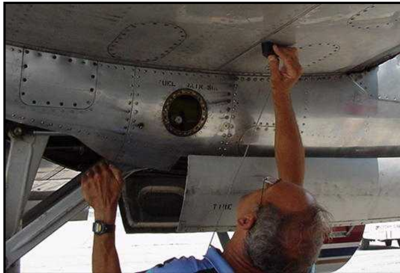
Field testing of eddy current inspection being completed on SA226 aircraft
