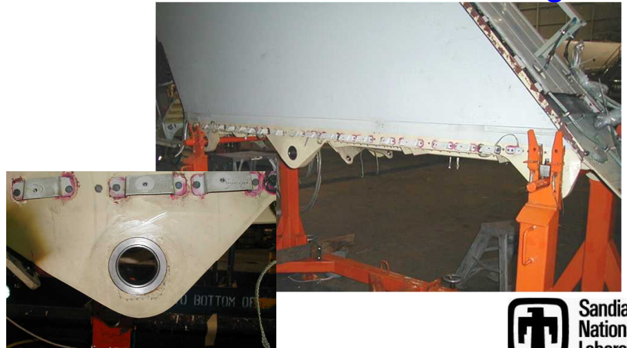
Developed P-E UT inspection – added for carbon laminate lug
