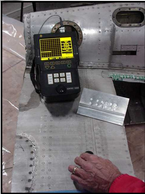
Inspection of lower wing spar testbed (Fairchild SA226)
