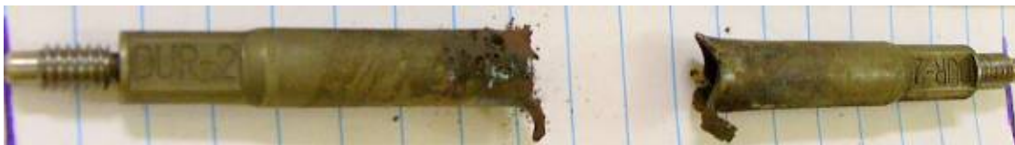
➔ post-test \text{DUO}_2 rodlet
