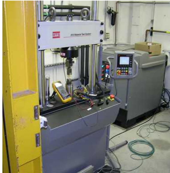
Figure 10 Mechanical test frame for dynamic loading of materials in high-pressure hydrogen gas.
